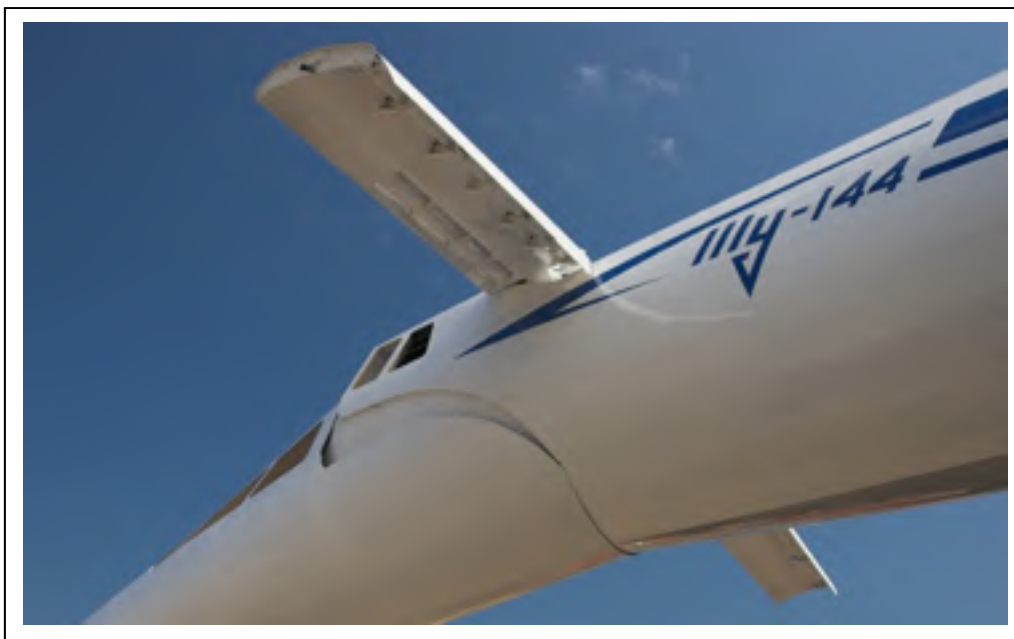
Figure 1.2 " Retractable foreplane of the Tupolev TU-144 " (cropped image) by Leonid Kruzhkov is licensed under CC BY-NC-ND 2.0 (taken from (Kruzhkov, 2007))
