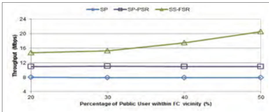
Figure 4.7 Throughput for the Variable FC User Density scenario, arrival rate equal to 16 MS/TU and 10% of FC subscribers
