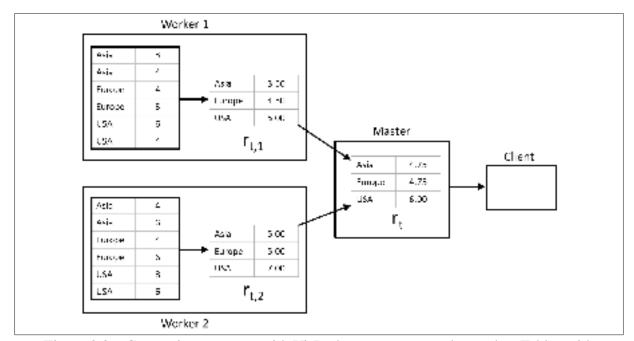
Figure 3.3 Computing averages with VisReduce over two worker nodes. Tables with thick borders may be very large, but do not leave the worker node they are stored on. Only relatively small amounts of data are transferred between nodes. At time t, each worker w produces result  $r_{t,w}$ ; the master node assembles these into result  $r_t$  to be displayed by the client. Specifically to compute averages, both the sum and the number of data points seen need to be tracked.
