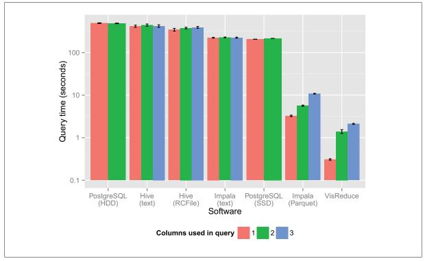
Figure 3.6 Log<sub>10</sub> plot of mean query completion time by query type. Error bars represent a 95% confidence interval for the mean. Queries on three columns for PostgreSQL were aborted after twenty minutes.
