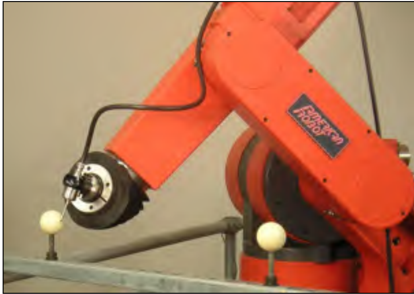
Figure 1.5 MasterCal calibration setup 5
