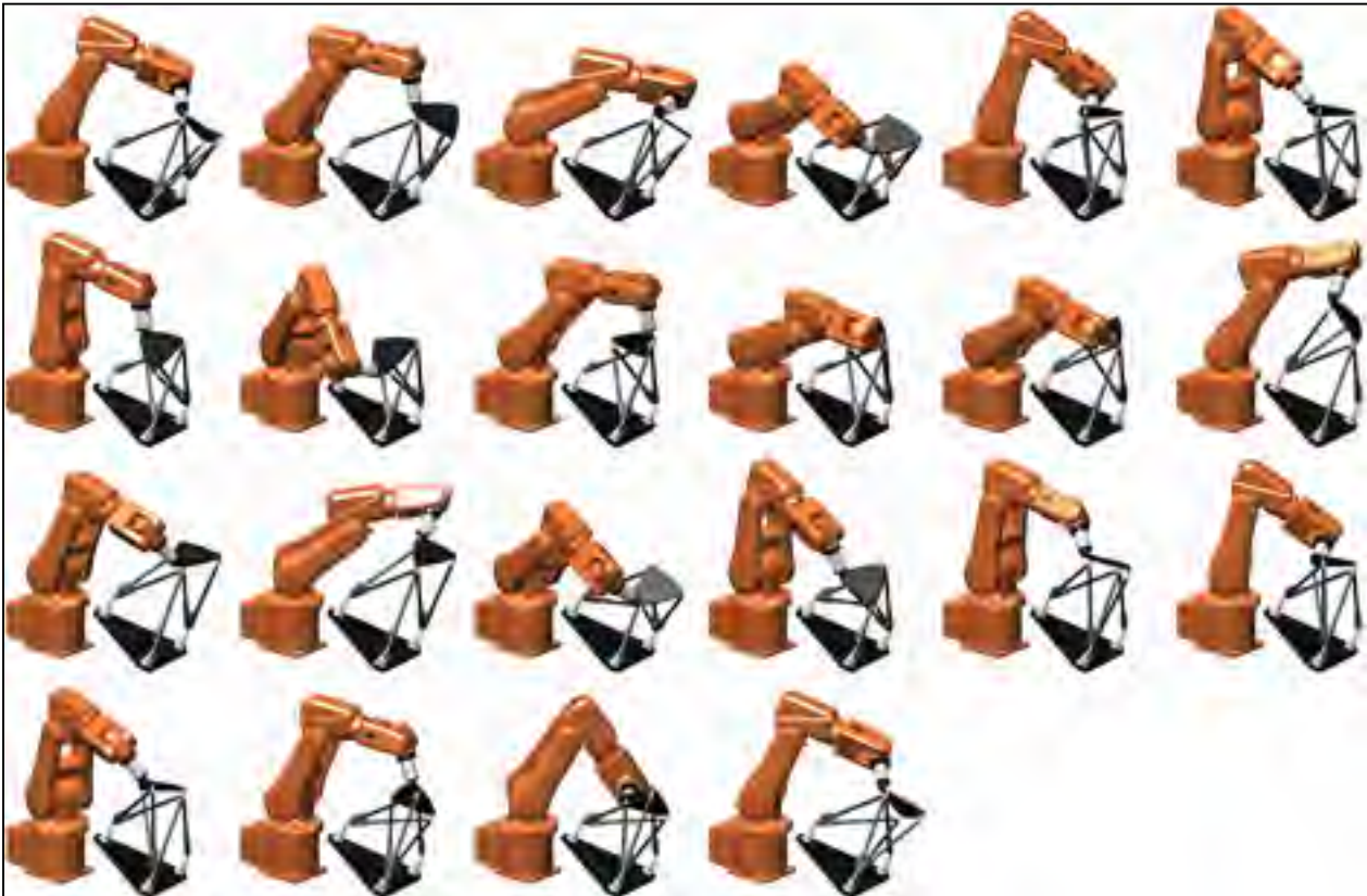
Figure 3.10 The 22 tool poses measurable using our device for a single setup of the base fixture. In 17 of these poses (not identified here), the robot can be positioned with two wrist configurations.
