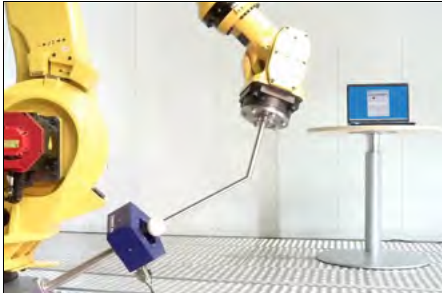
Figure 1.4 Robot calibration using LaserLAB 4
