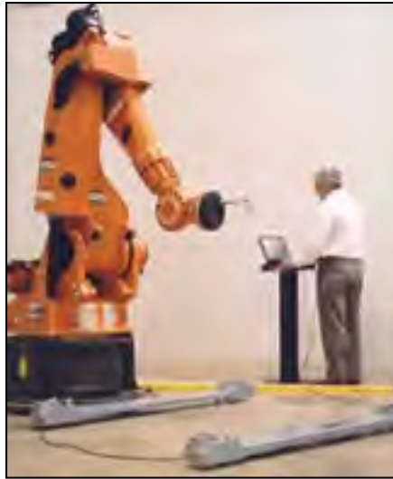
Figure 1.1 Robot calibration using the CompuGauge device 1
