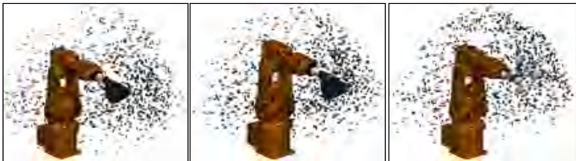
(a) (b) (c) Figure 2.7 Calibration and validation positions using (a) the laser tracker and the triangular artifact (setup 1); (b) the C-Track and the triangular artifact (setup 2); (c) the C-Track and the spatial artifact (setup 3)
