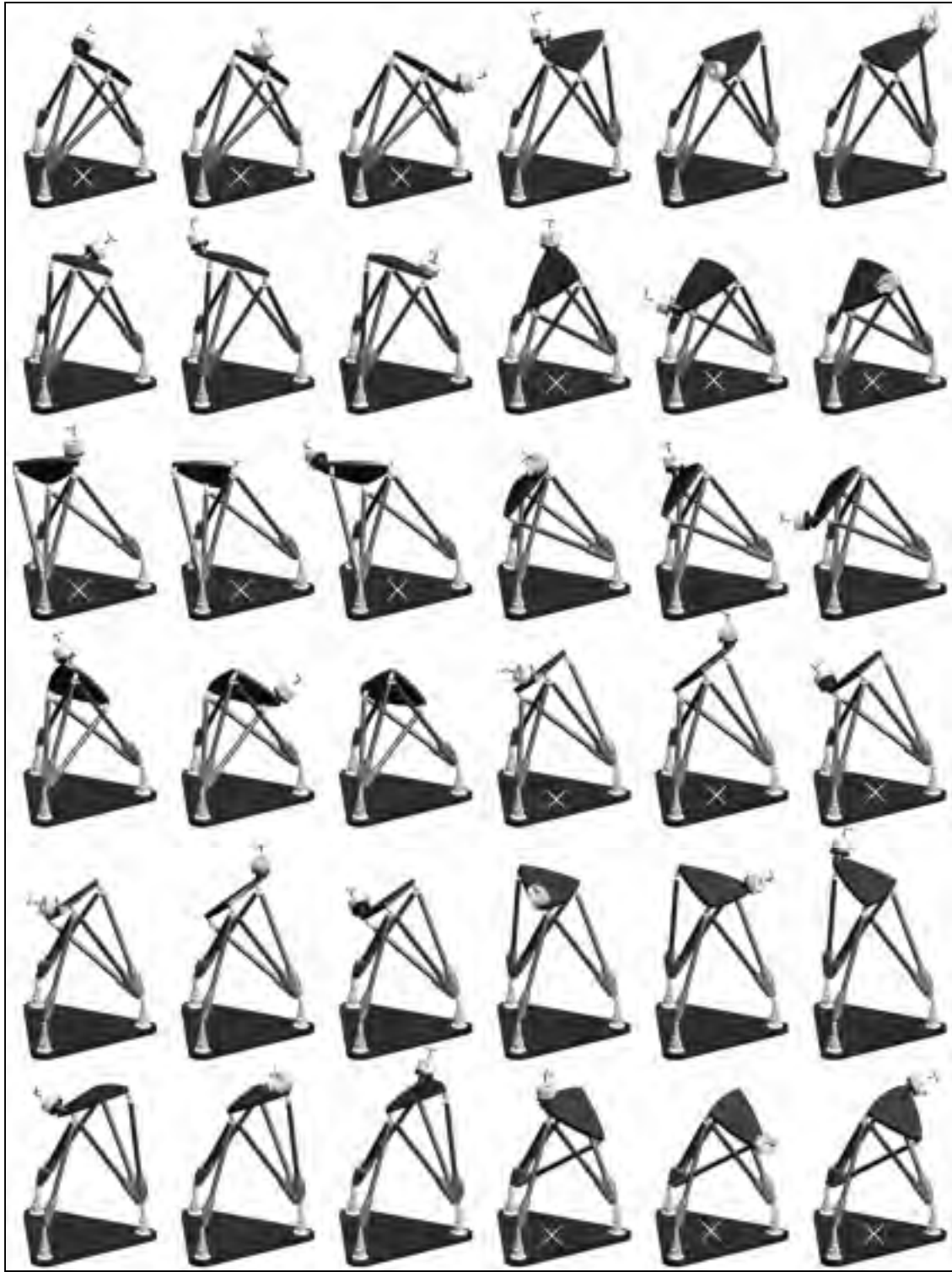
Figure 3.6 The 72 different tool poses that can be measured using our device (18 of these, marked with a white cross, are superfluous)
