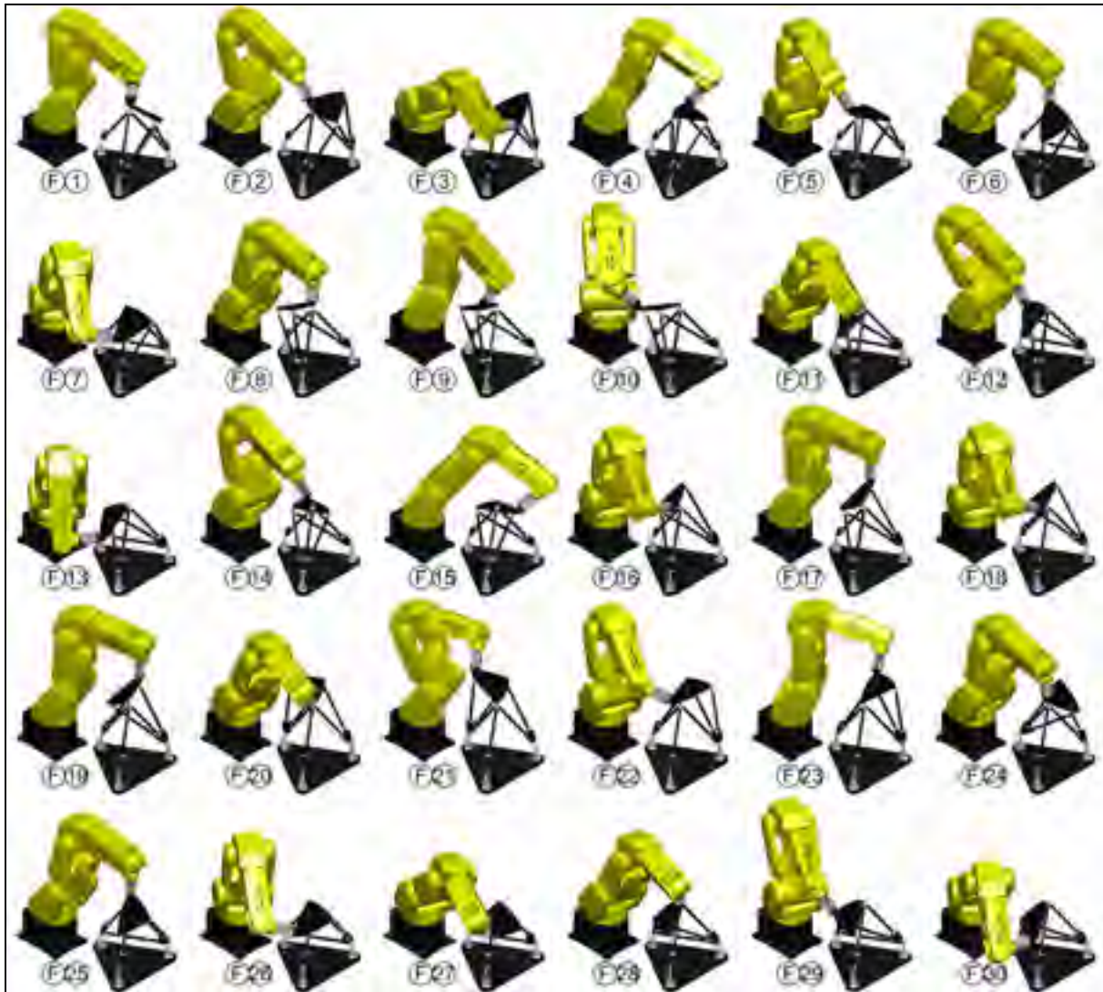
Figure 4.6 Robot configurations used for calibration (continues)
