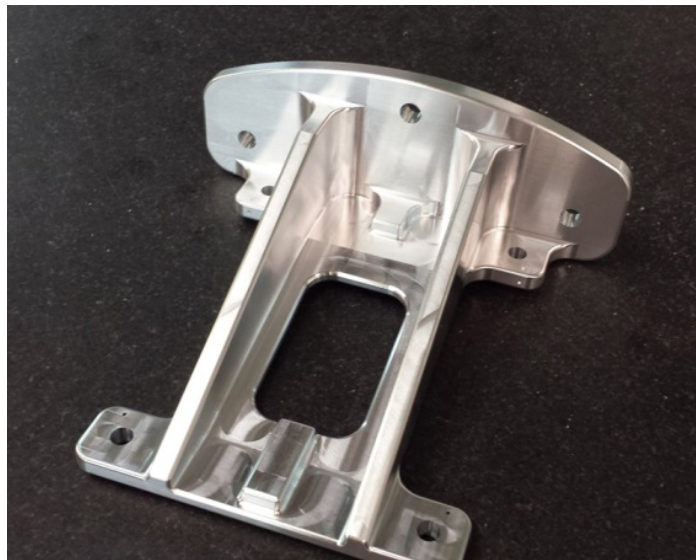
Figure 1-18 Precision CNC Machining of 6061-T651 aluminum Brackets (courtesy of EMF Inc.)
