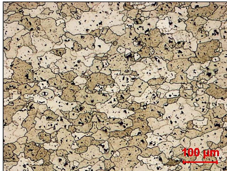
Figure 2-1 Optical microstructure of the aluminum AA7075-T651 alloy.
