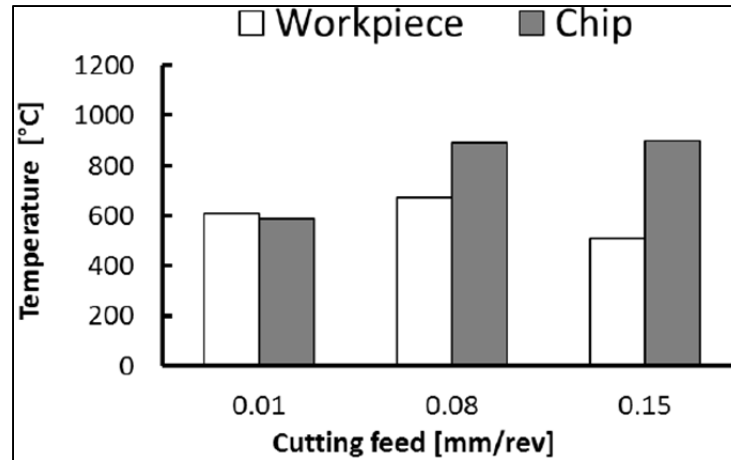
Figure 3-27 Effect of cutting feed on the workpiece and chip temperatures for V=128 m/min and DOC=0.5 mm
