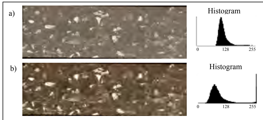
Figure 3-6 Optical image enhancement through histogram stretching, (a) raw image, (b) after stretching
