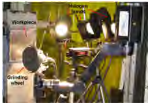
Figure A I-1 High speed camera setup used for observation of impact cutting
