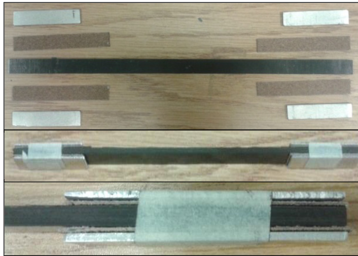
Figure 2.6: Sample with sandpaper and aluminium tabs
