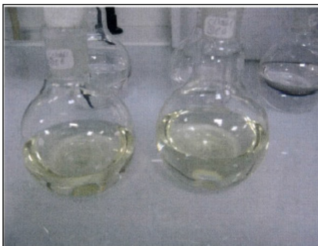
Figure 3.17 Extraction type Soxhlet teneur en extractibles
