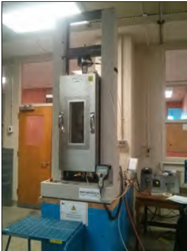
Figure 3.4 : Machine de traction MTS Insight
