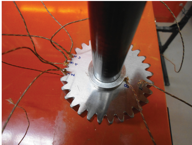
FIGURE A.6 – Placement des thermocouples.
