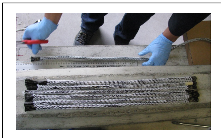
Figure 7.1 Preparation of CFRP ropes into desired lengths
