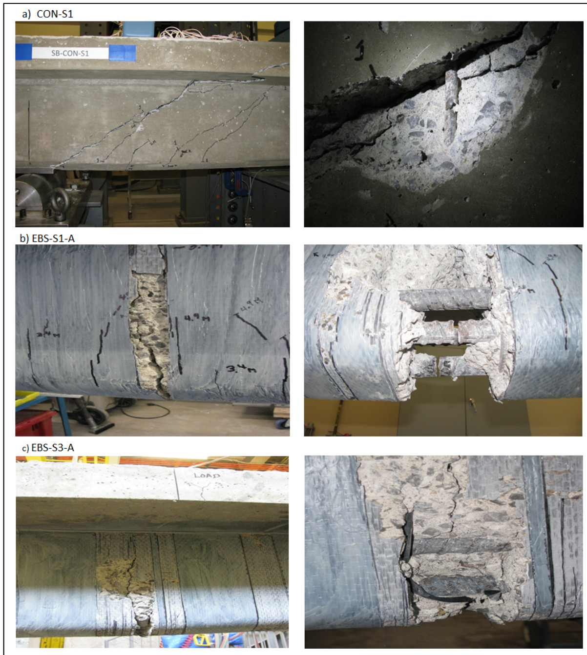
Figure 4.3 Crack pattern at failure and steel rupture under fatigue loading: a) CON-S1; b) EBS-S1-A; c) EBS-S3-A
