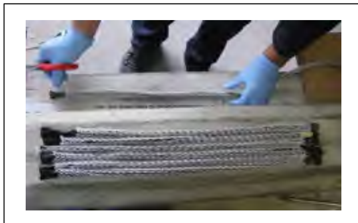
Figure 7.1 Preparation of CFRP ropes into desired lengths
