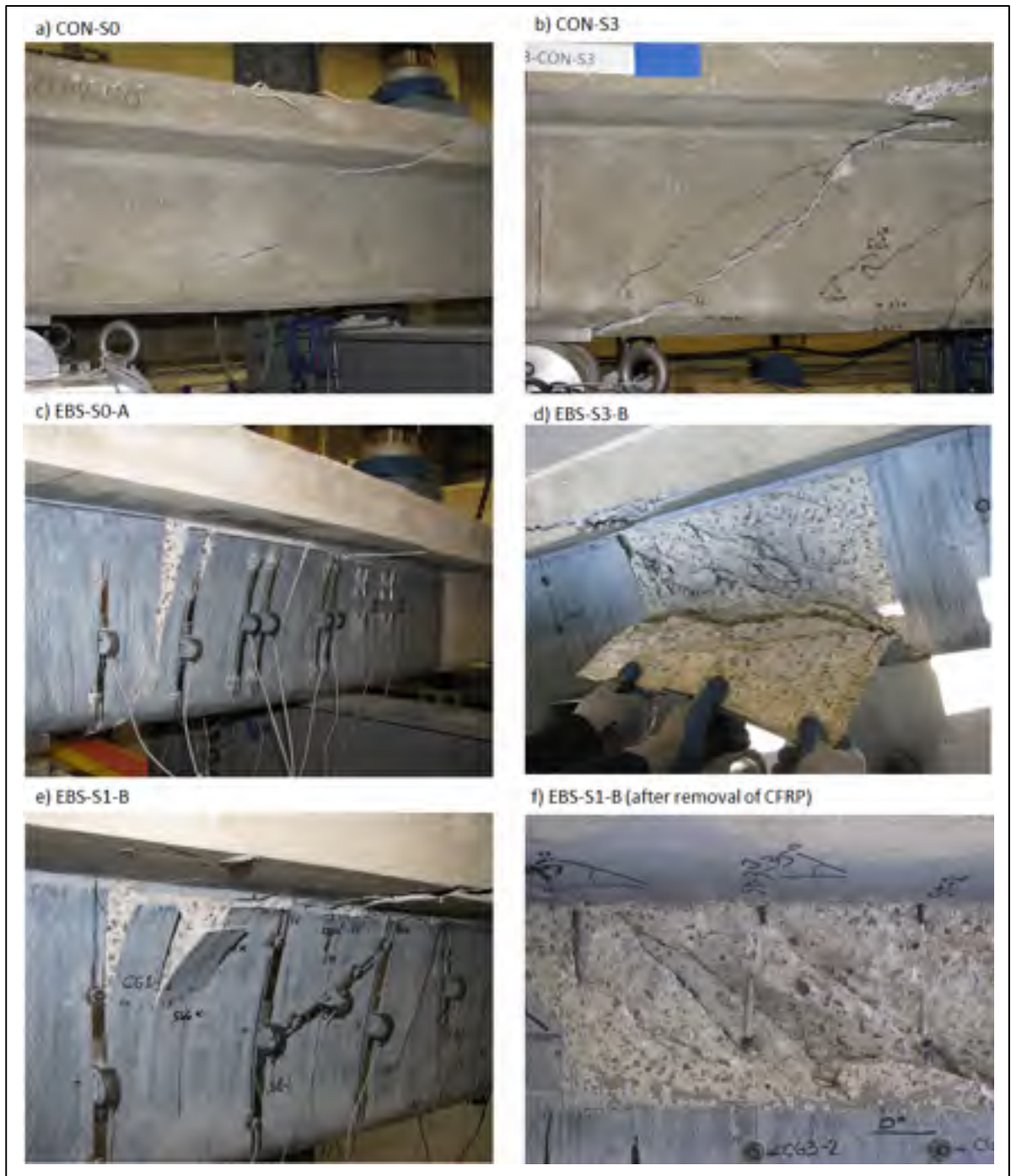
Figure 4.4 Common failure mode under monotonic loading: a) CON-S0; b) CON-S3; c) EBS-S0-A; d) EBS-S3-B; e&f) EBS-S1-B before and after removal of FRP sheet
