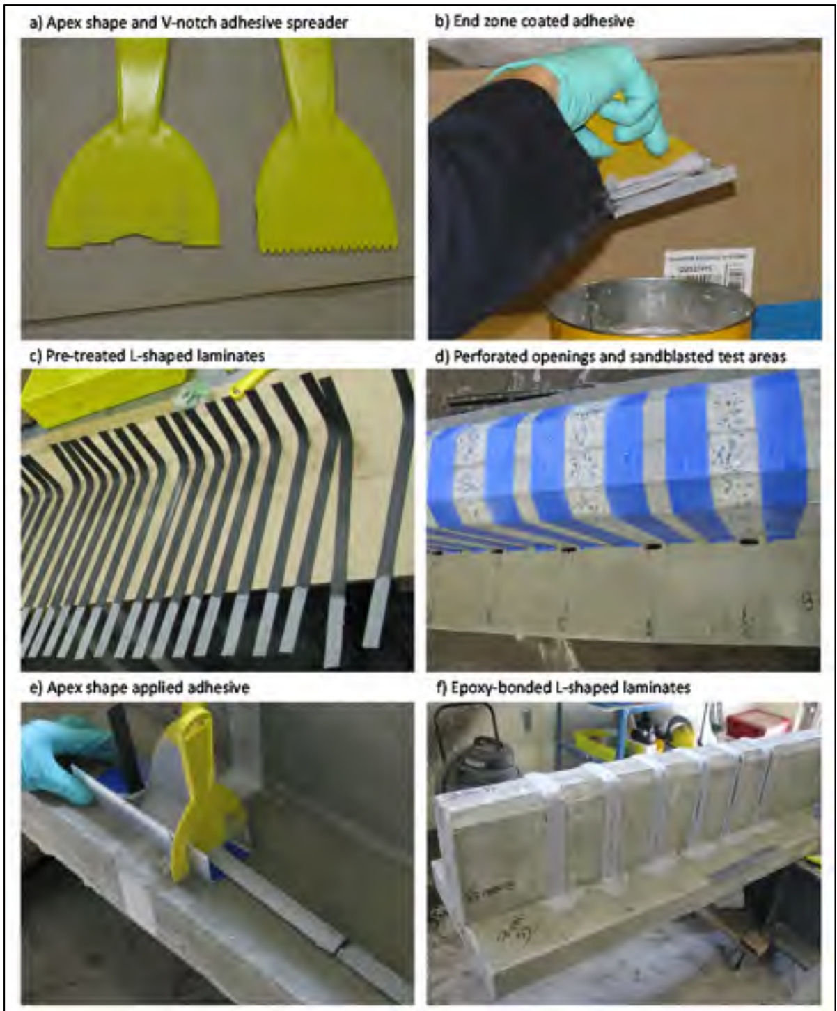
Figure 5.2 Step-by-step procedure for CFRP L-shaped laminates application
