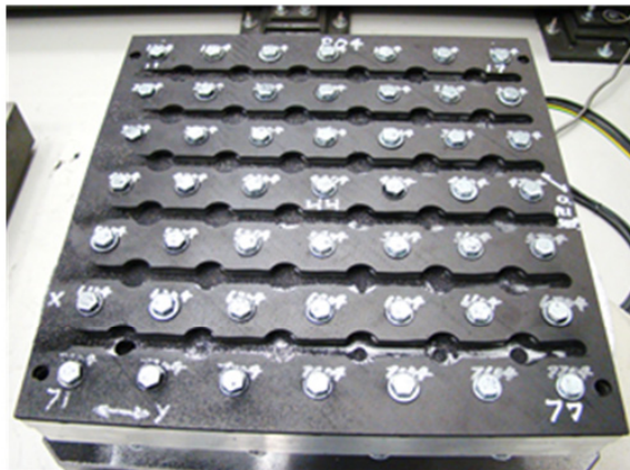
b) Semi-Finished part after trimming of the 42 slots in OP1 operation
