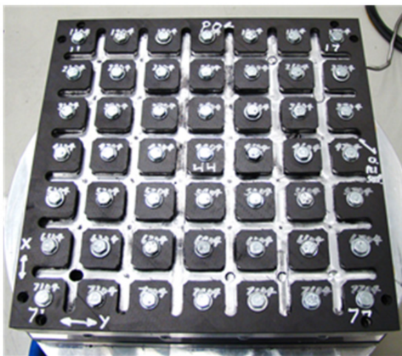
c) Finished part after trimming of the 84 slots in OP1 and OP2 operations
