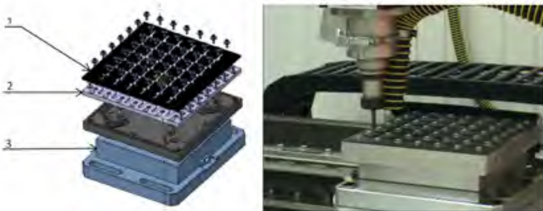
Fig.6 Experimental setup for trimming of CFRP
