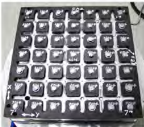
c) Finished part after trimming of the 84 slots in OP1 and OP2 operations
