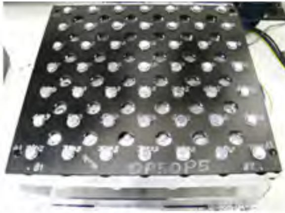
a) Rough part before trimming of the 48 slots
