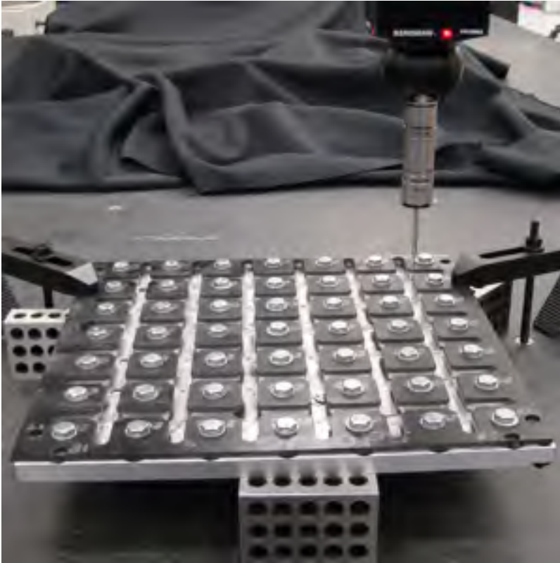
Fig.15 Inspection of the trimmed specimens
