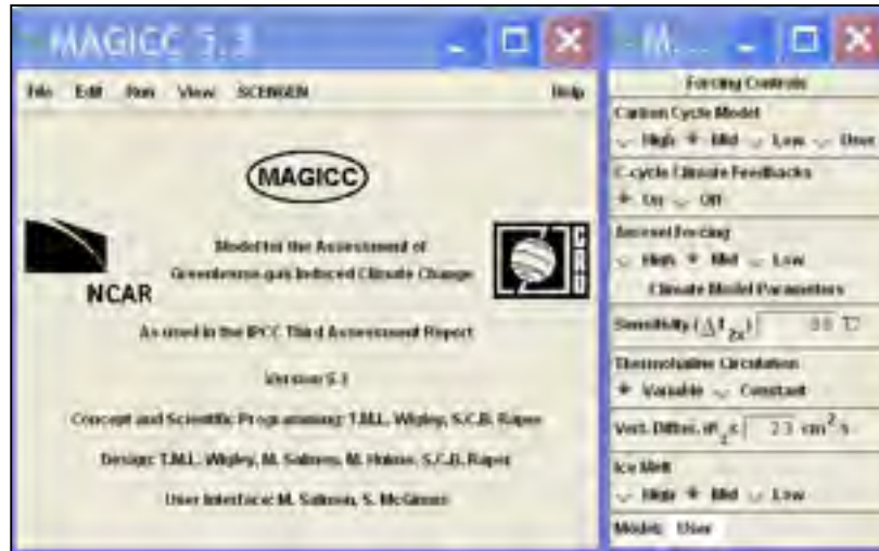
Figure 3.3 Adjustable forcing controls and climate model parameters in the MAGICC model
