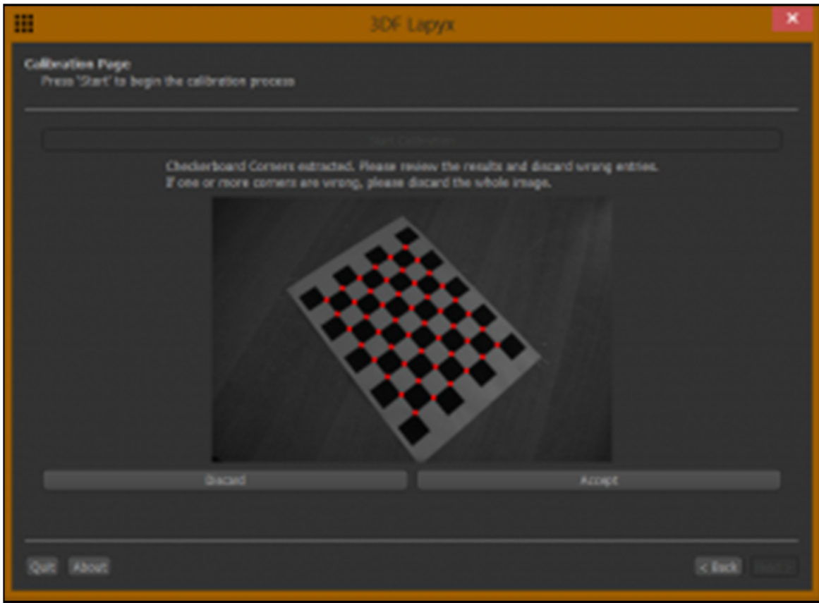
Figure 3.12: 3DF Lapyx automatic camera calibration software that extracts the typical intrinsic camera parameters used in Computer Vision
