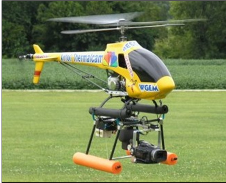
Figure 3.27: Remote controlled Helicopter for WT image acquisition (Source: http://www.airfoilskeycam.com )
