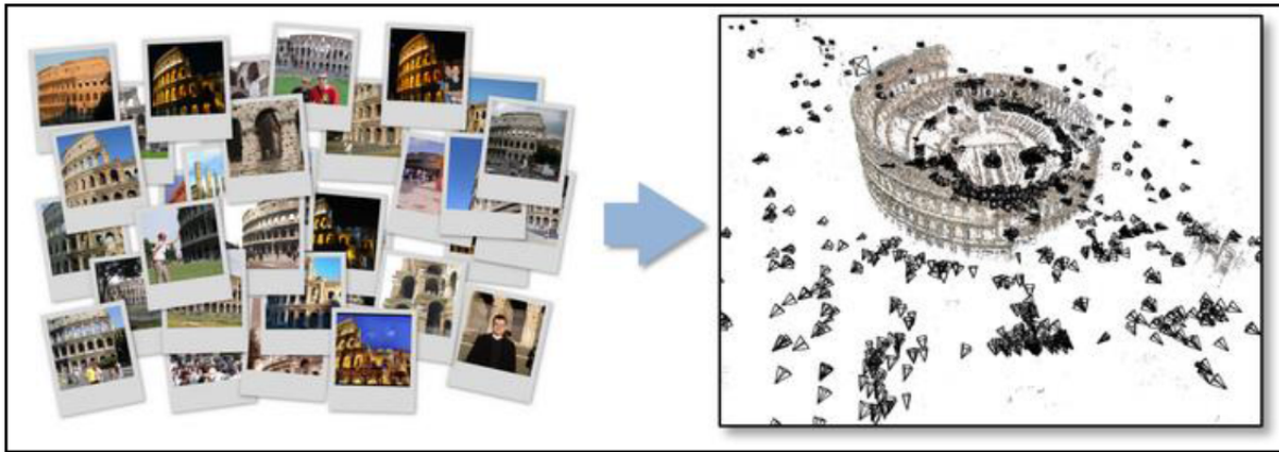
Figure A. 17: Brief example of the use of Bundler: Structure from Motion (SfM) (Snavely, 2010)
