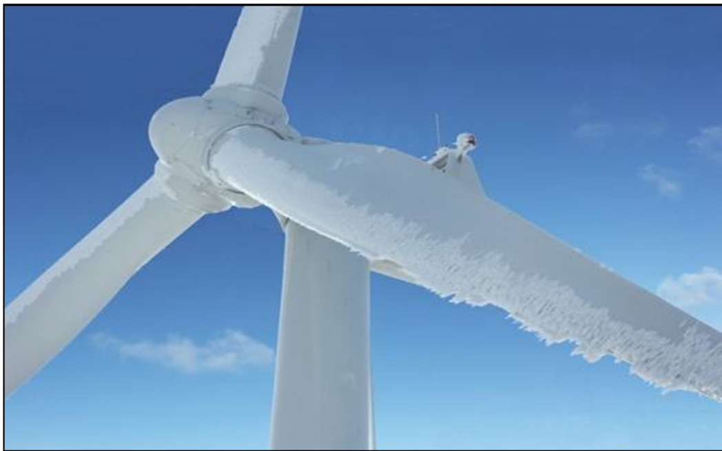
Figure 1.2: Problematic ice vanes on the windward side of the blade
