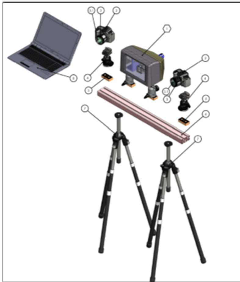
Figure A. 8: Ice Measurement Laser Scanner Exploded View of Components
