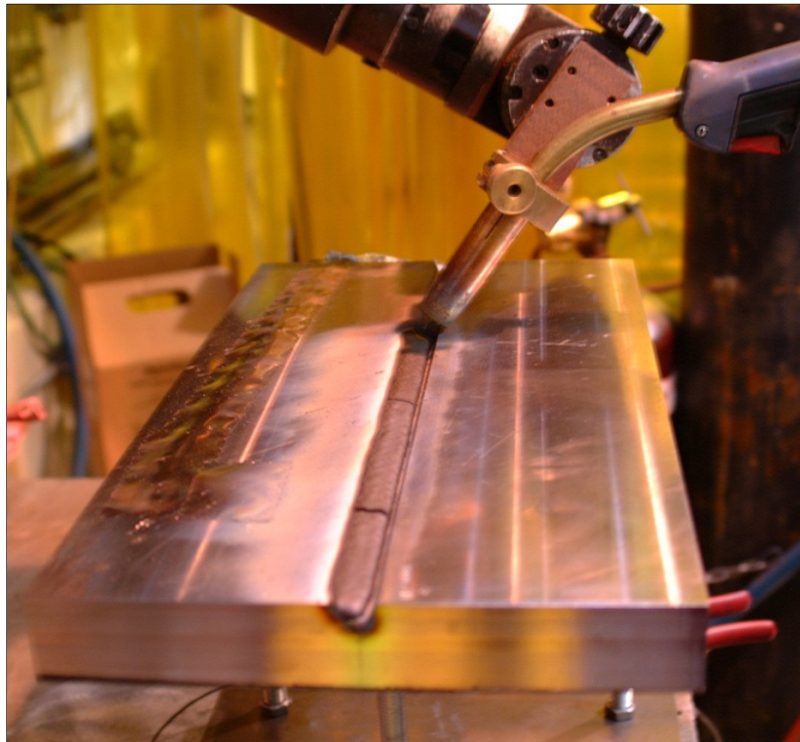
Figure 3.11 Installation of the plate and angle of torch for second pass of welding
