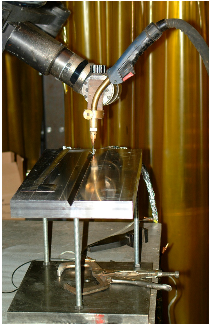
Figure 3.8 Installation of the plate on three points
