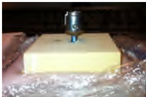
Figure 1. Pedicle screw has been fully inserted into polyurethane foam specimens
