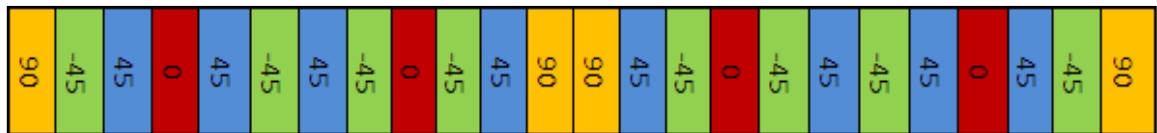
Figure 2.5 Stacking sequence of CFRP laminate
