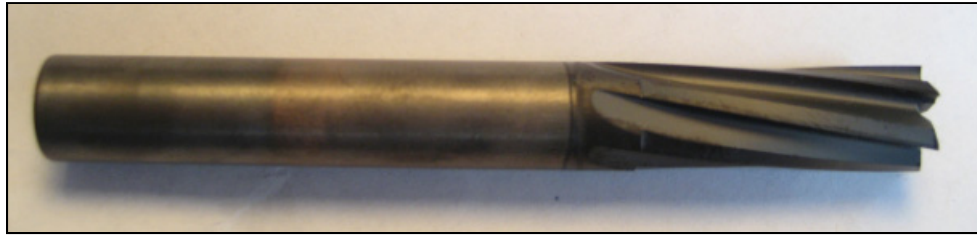
Figure 2.4 CVD coated cutting tool
