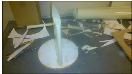
Figure 8. Embedded airfoil on the support disc.
