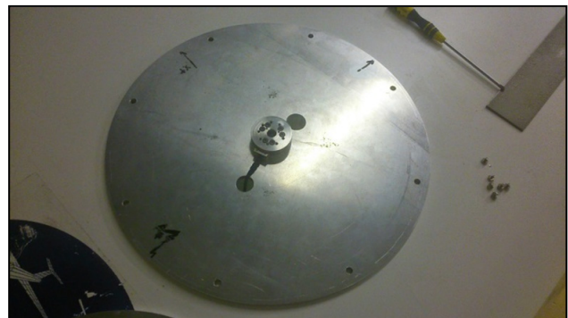
Figure 5. ATI sensor fixed on the aluminum plate.
