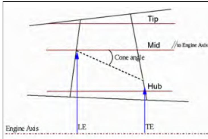
Figure 2.1 Cone angle definition
