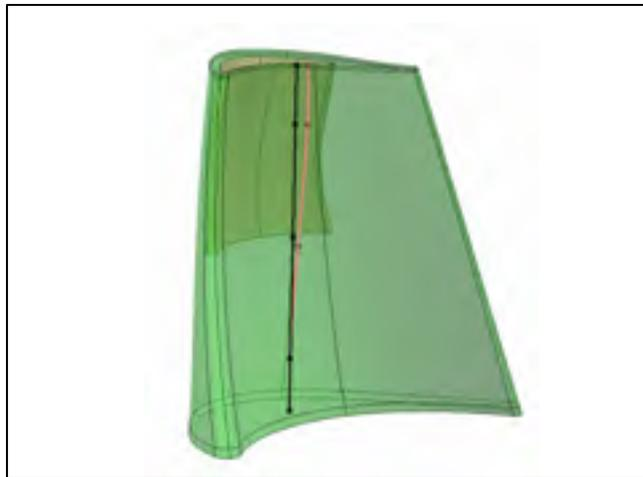
Figure 3.5 Corrected stacking for airfoils with cavity
