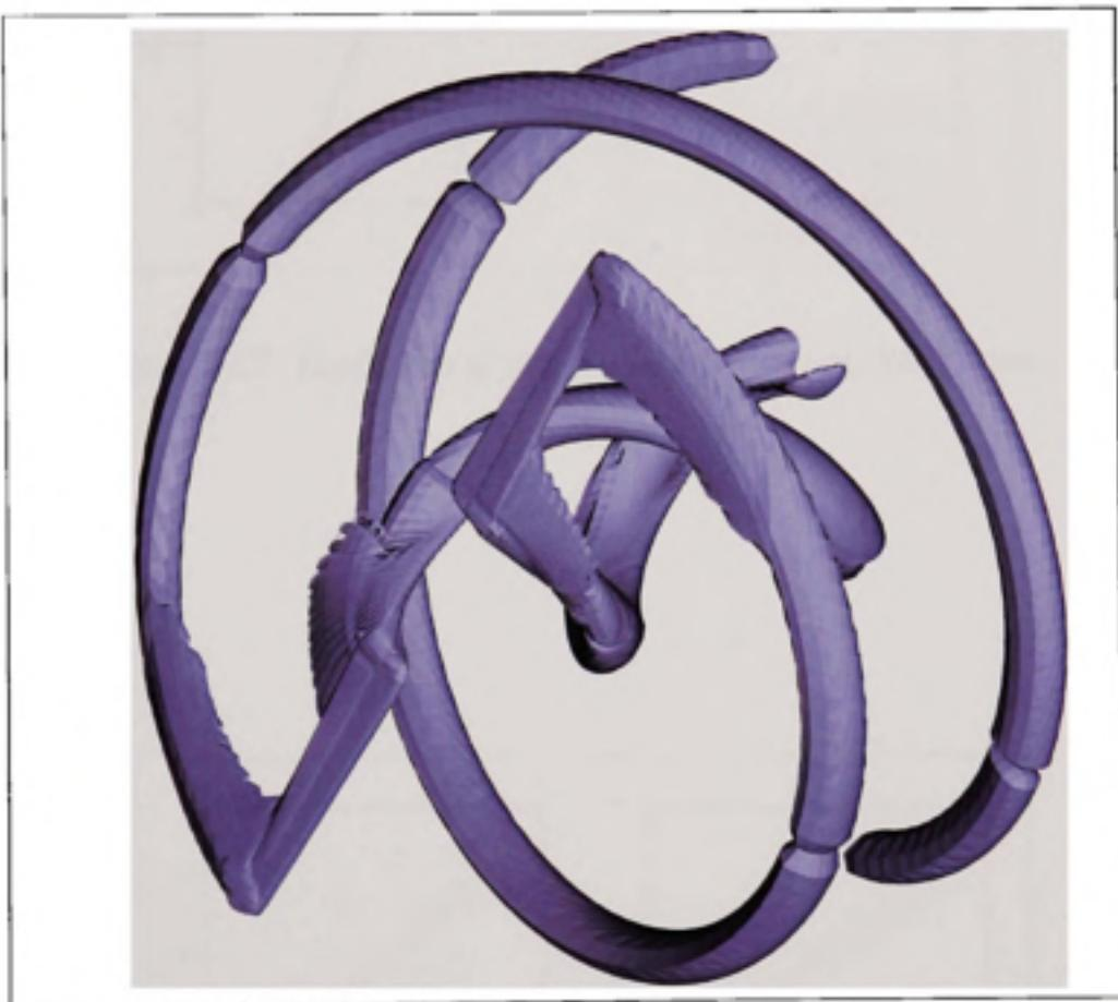
Figure III.6 Isosurfaces of vorticity for the NREL rotor,  $\lambda = 4$ , NS-AS model.
