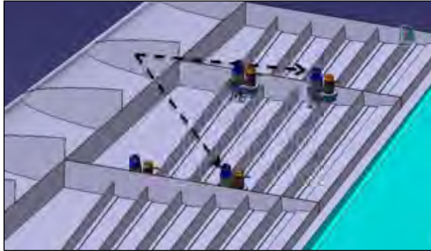
Figure 2.2 Overview of the morphing mechanism without the upper skin
