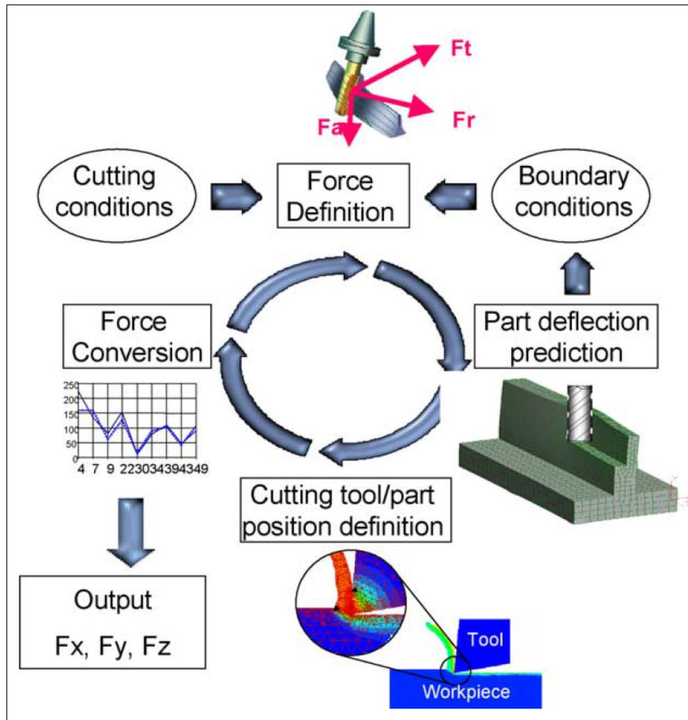
Figure 1.5. Iterative flexible force prediction model
