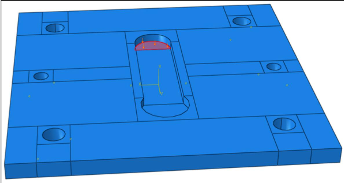
Figure 2.10. Area of the acting cutting force  $F_z$
