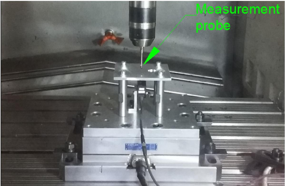
Figure 4.3. Identification of the reference point for the depth of cut during machining
