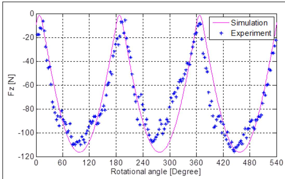
Figure 2.7. Comparison of axial cutting force (6111 RPM, 0.127 mm/tooth)
