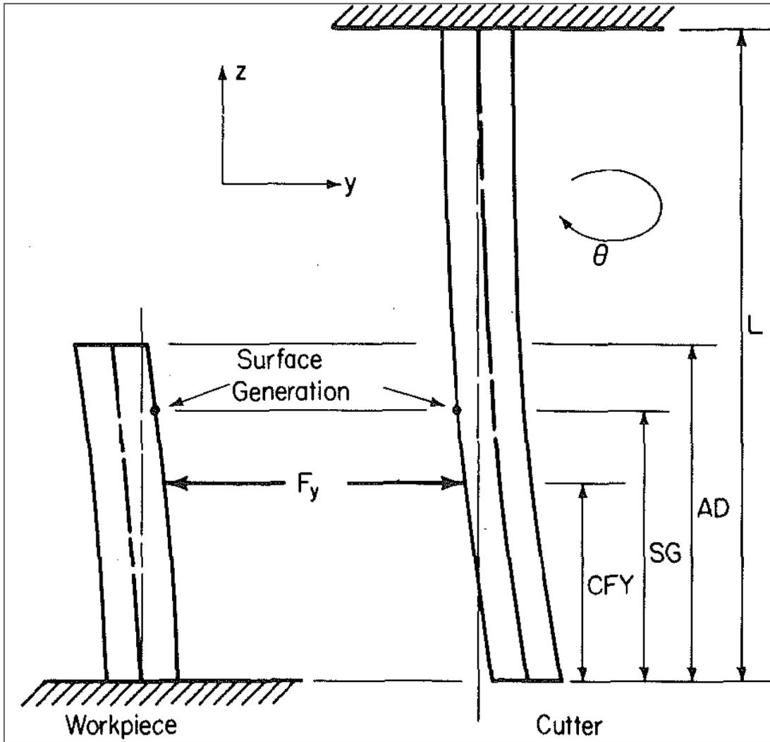
Figure 1.4. Cutter and workpiece deflections (Kline et al., 1982)
