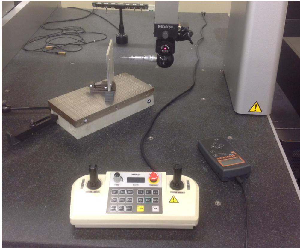
Figure 3.2. CMM measurement of the thin plates
