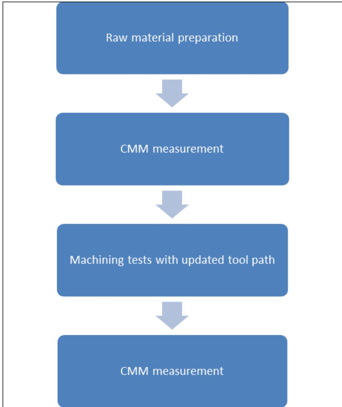
Figure 5.2. Experimental process with cutting errors compensation
