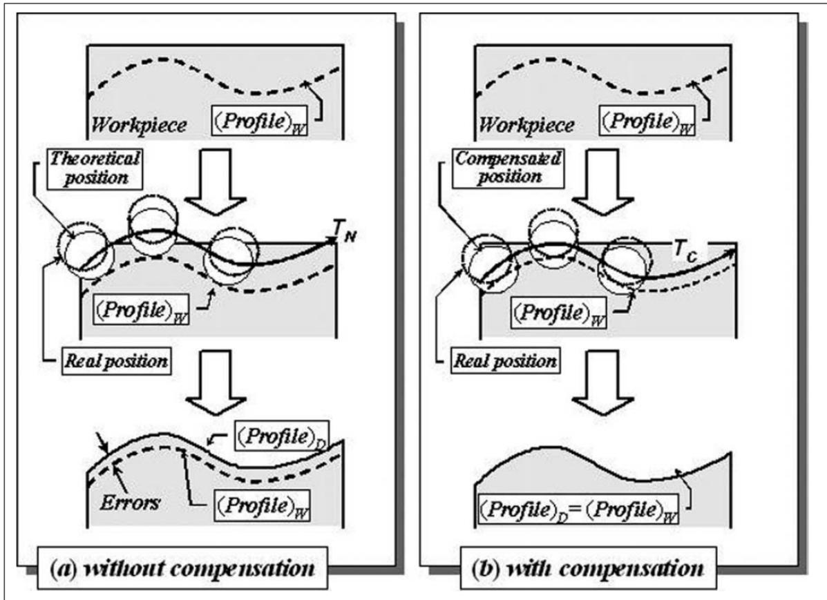
Figure 1.9. Path compensation (Dépincé and Hascoët, 2006)
