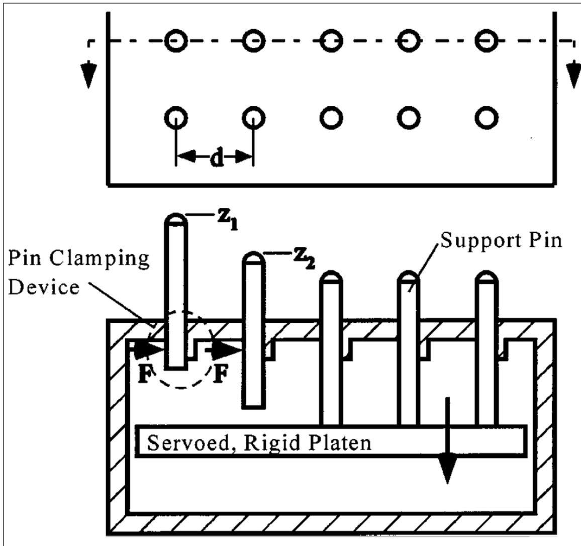
Figure 1.3. RFD concept diagram shown in pin setting mode (Walczyk and Longtin, 1999)
