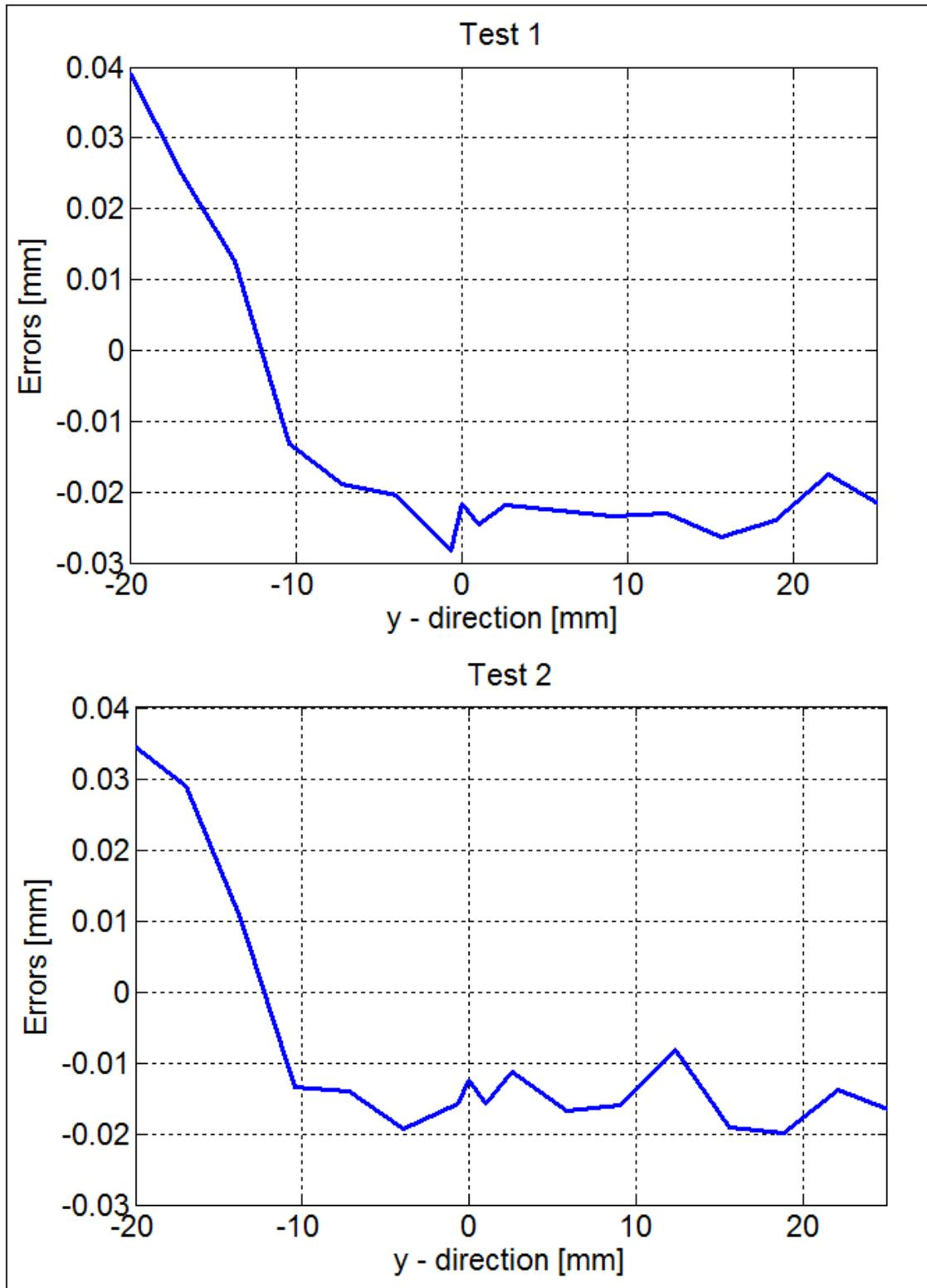
Figure 5.3. Cutting errors of machined workpieces after machining processes with compensations (Test 1 and Test 2)
