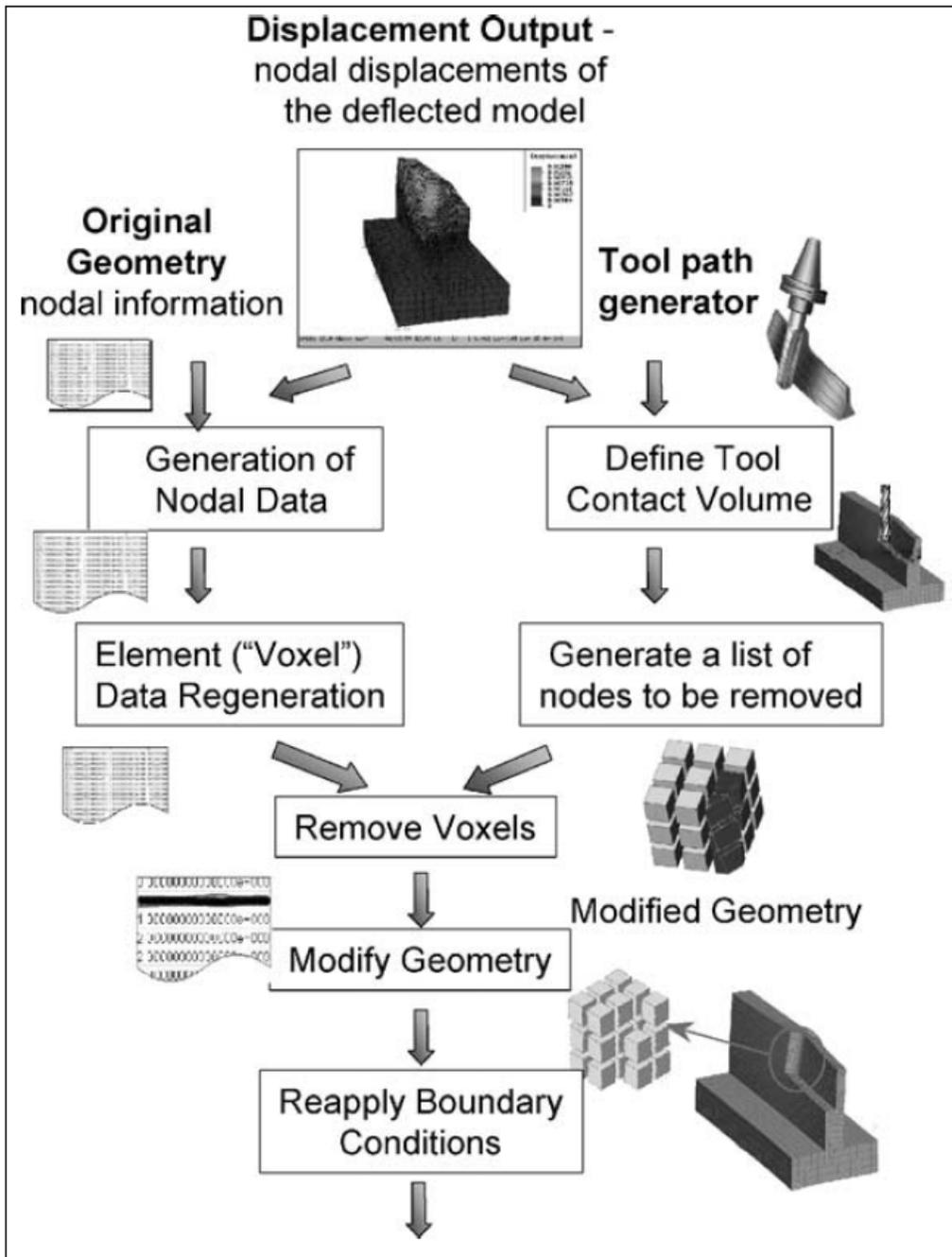
Figure 1.6. Voxel-based modelling for error prediction and compensation (Ratchev et al., 2003).
