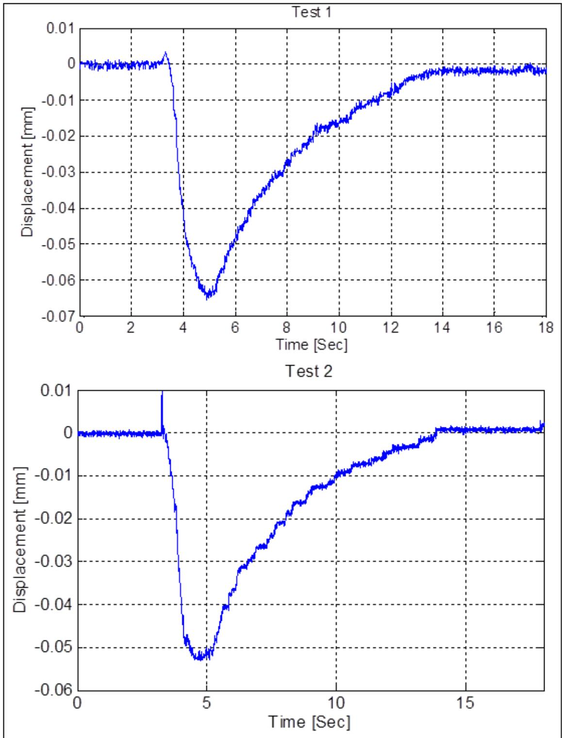
Figure 4.2. Displacement of central points in different tests (Test 1 and Test 2)
