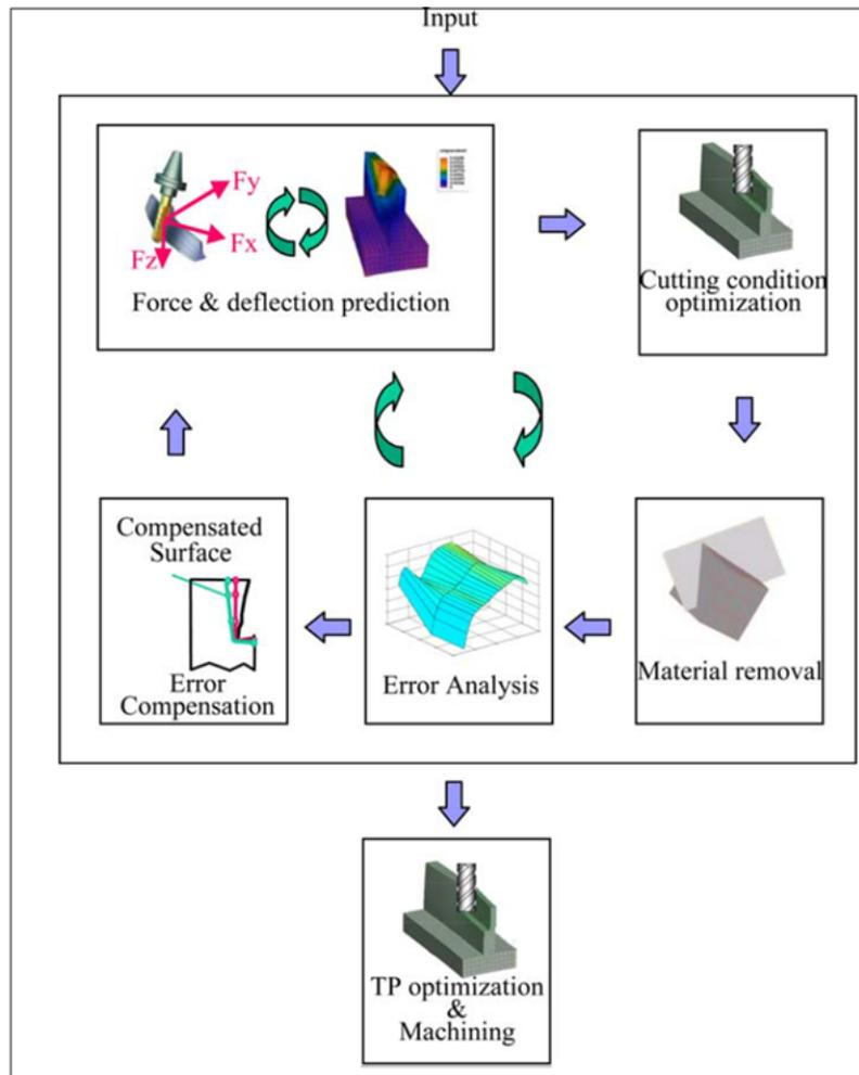
Figure 1.7. An adaptive machining environment methodology overview (Ratchev et al., 2006)
