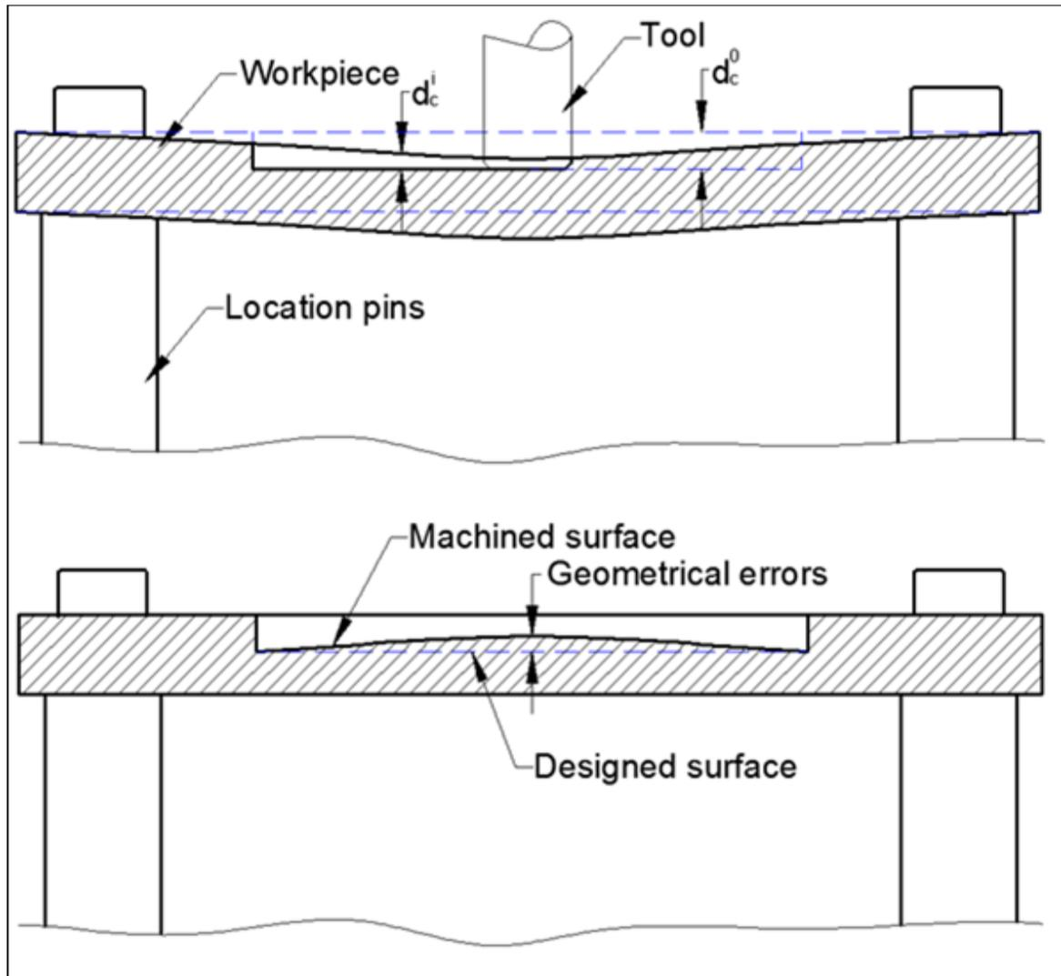
Figure 2.2. Material deformation during machining and geometrical profile after machining
