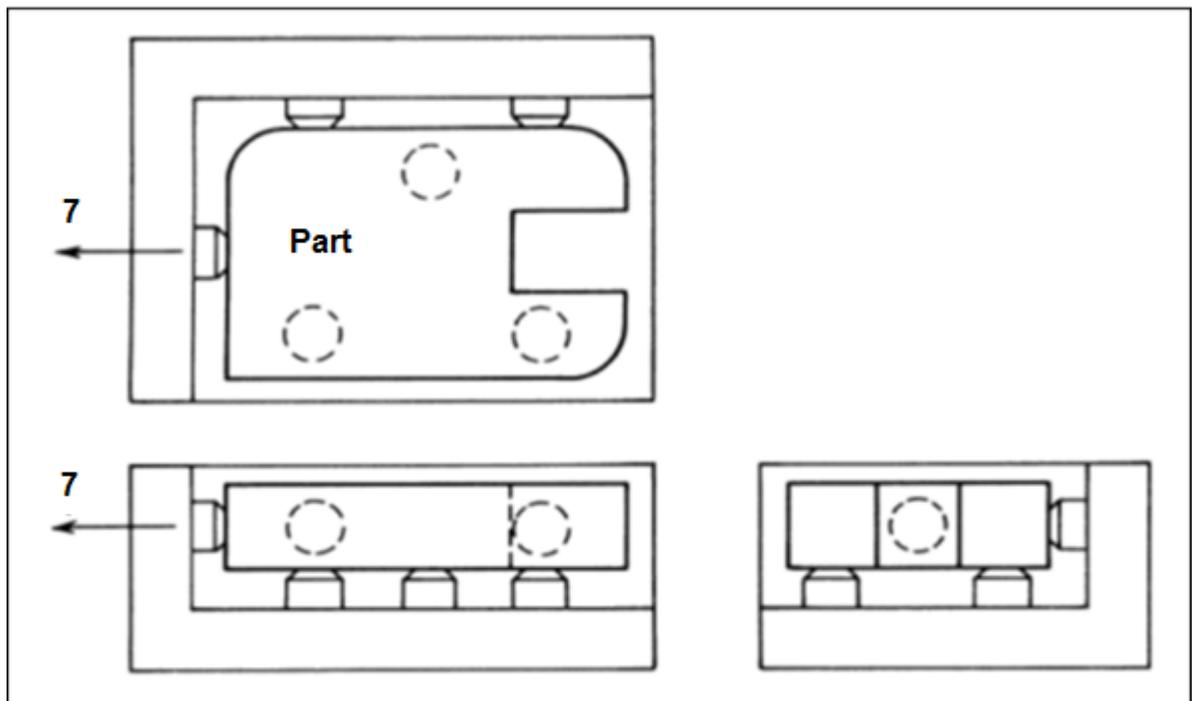
Figure 1.1. 3 – 2 – 1 principle (Foster, 1982)
