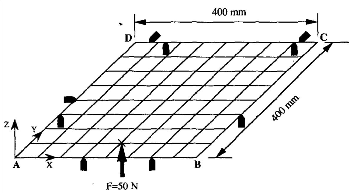
Figure 1.2. An example of system with N-2-1 principle,  $N = 6$  (Cai et al., 1996)
