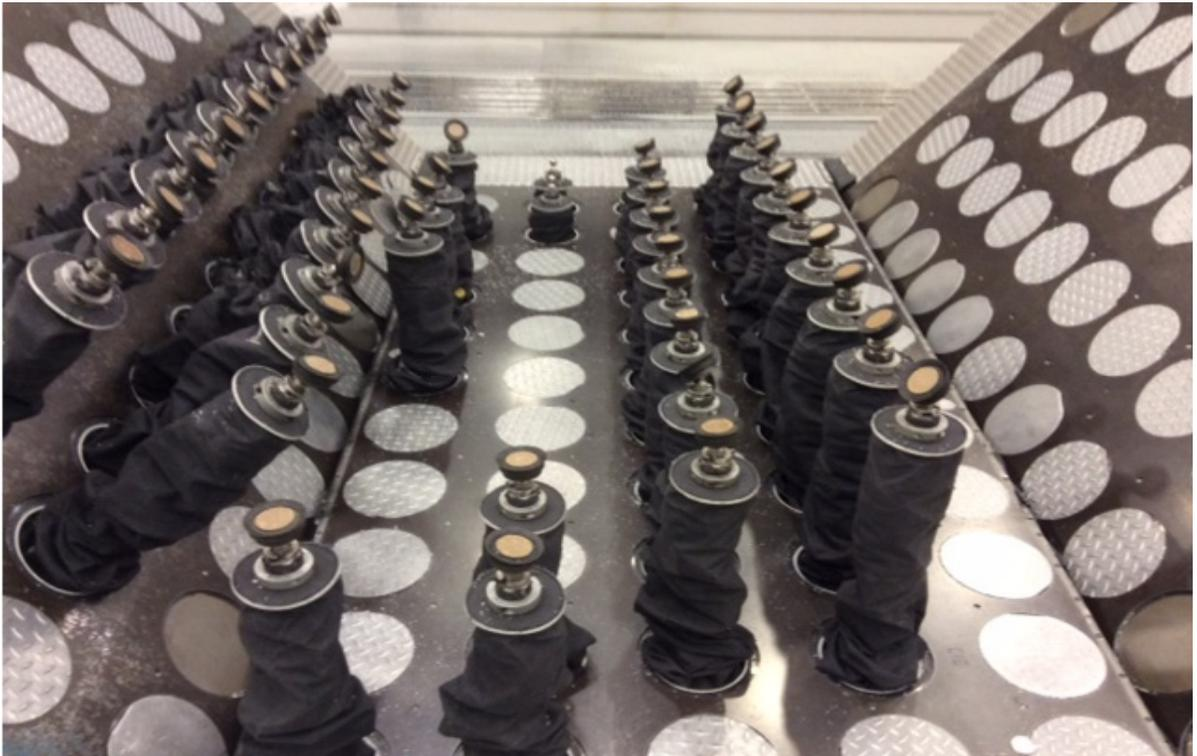
Figure 0. 1. Fixture with support pins on bottom face of the workpiece in the industry
