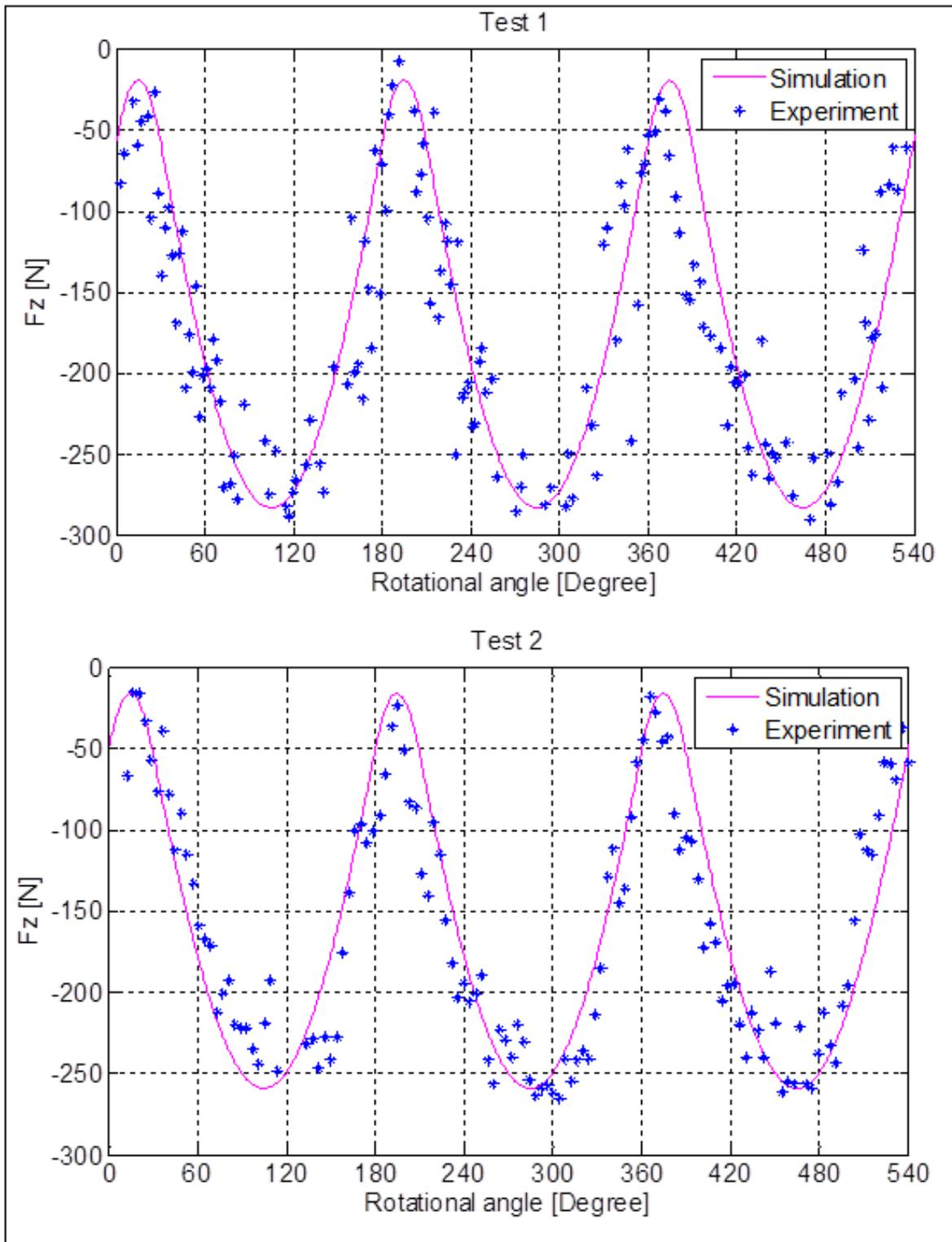
Figure 4.1. Cutting force in z-direction (Test 1 and Test 2)
