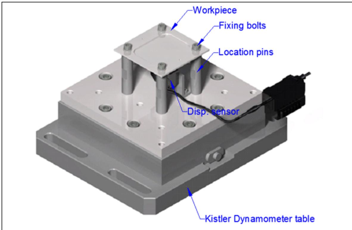
Figure 2.1. Flexible setup design
