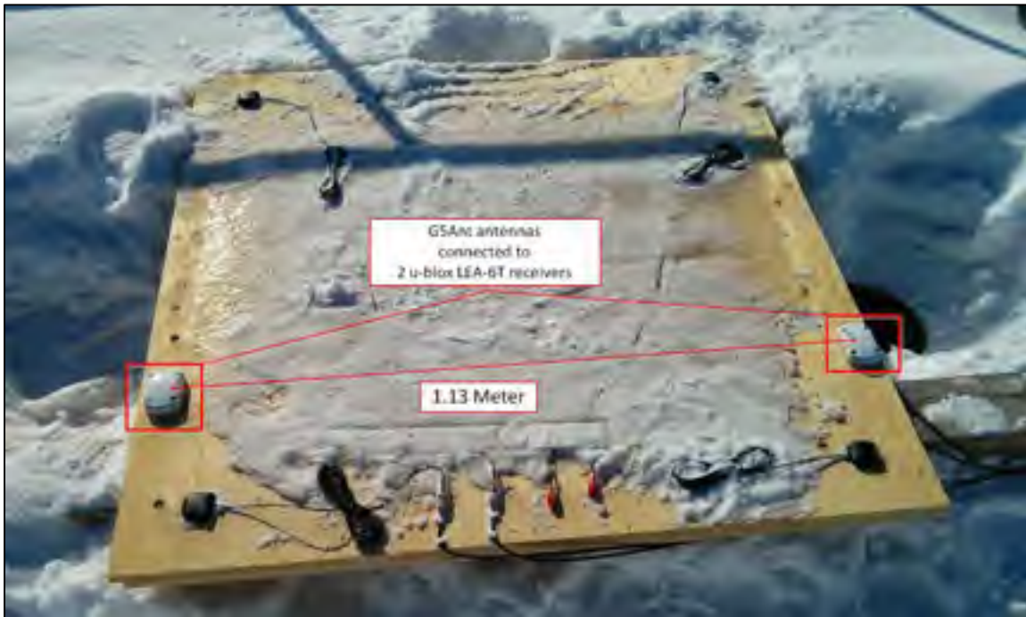
Figure 5.21 Data record configuration with two u-blox LEA-6T and two G5Ant-4AT1
