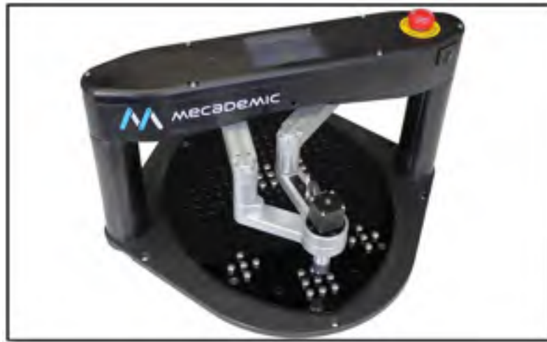
Figure 1.2 DexTar Robot; an example of parallel robot Taken from Bonev (2013)
