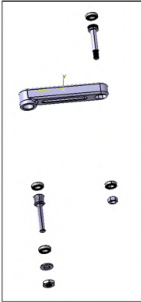
Figure 3.2 Exploded view of parts for the third link subassembly
