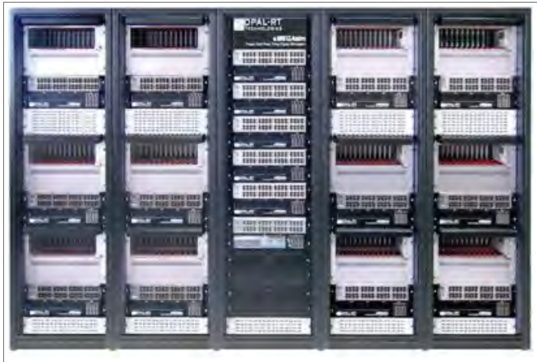
Figure 1.14 Real-time simulator with IOs chassis
