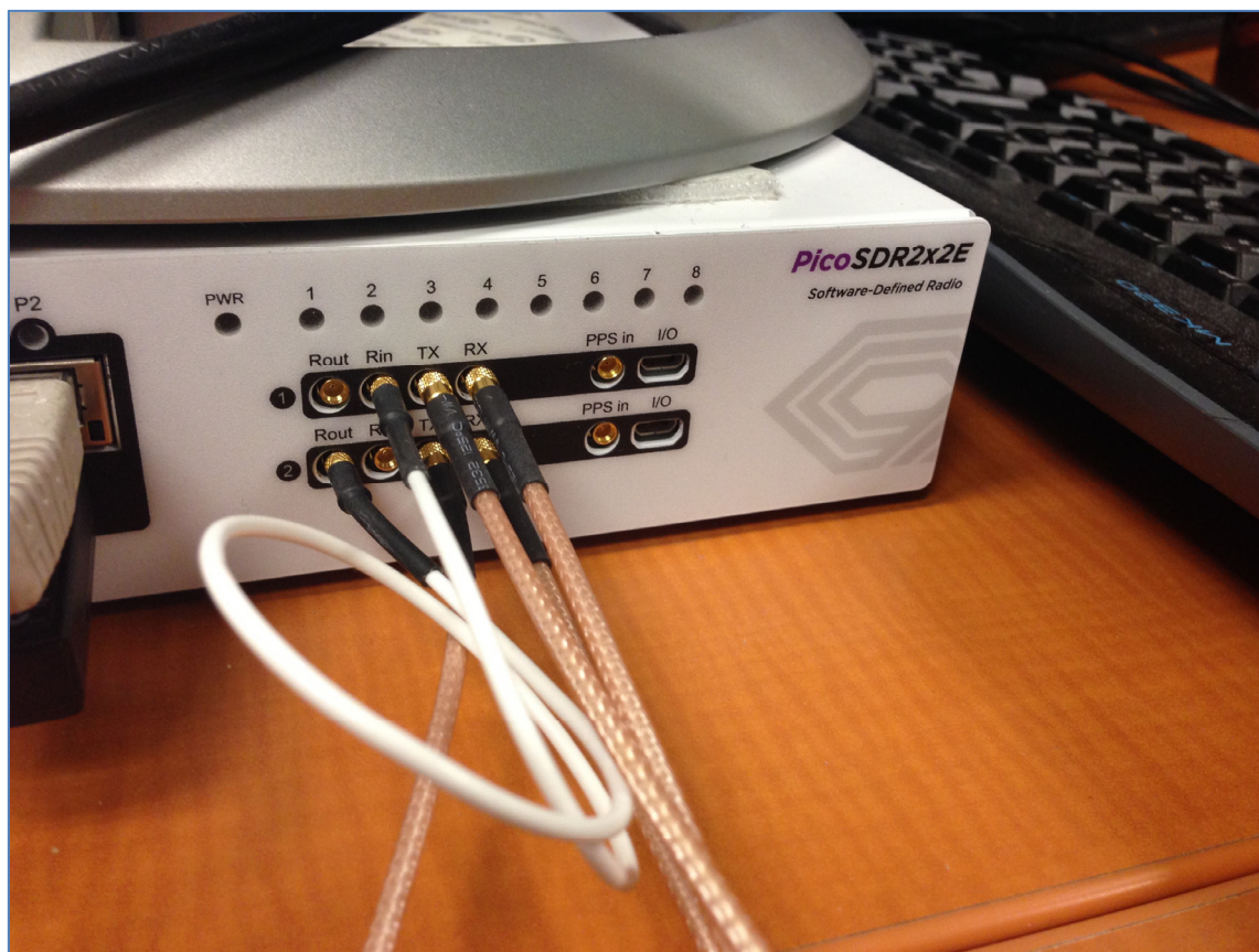
Figure 4.16 Radio 1 Reference-In Connected to Radio 2 Reference-Out (White cable)
