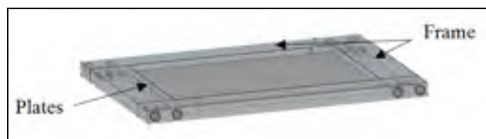
Figure 2.28 CAD of flat mould Taken from Roy (2014)
