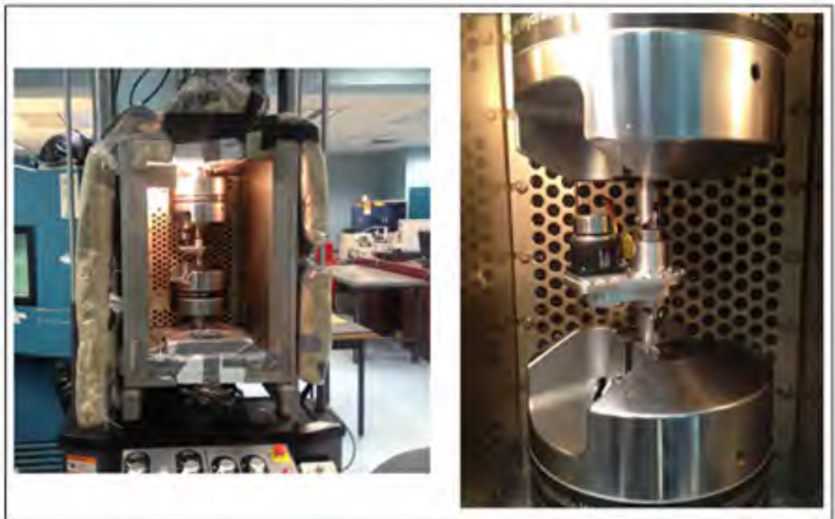
Figure 1.2 Actuator during robustness test at the ETS
