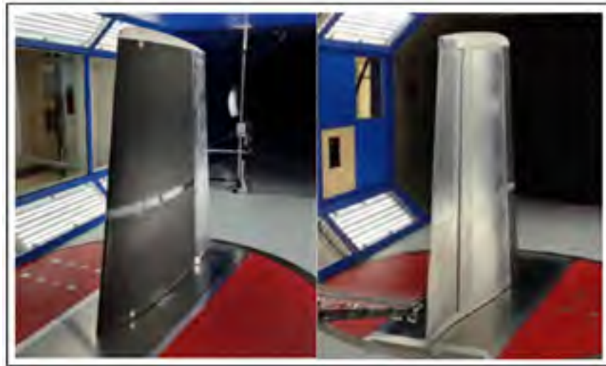
Figure 6.18 MDO 505 wing model setup in wind tunnel tests
