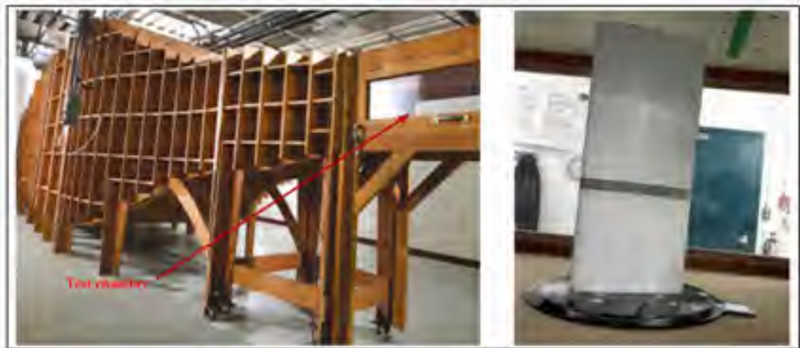
Figure 3.10 LARCASE Price- Païdoussis subsonic blow down wind tunnel and the morphing wing positioning in the test chamber
