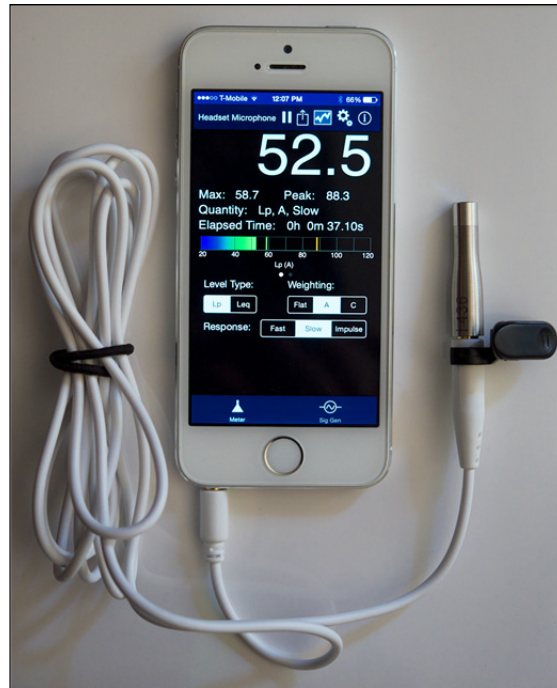
Figure 2.17 Replicating a shoulder-worn dosimeter, using the iPhone 5S running Faber Acoustical SoundMeter with the MicW i436 including extension cable and clip accessories
