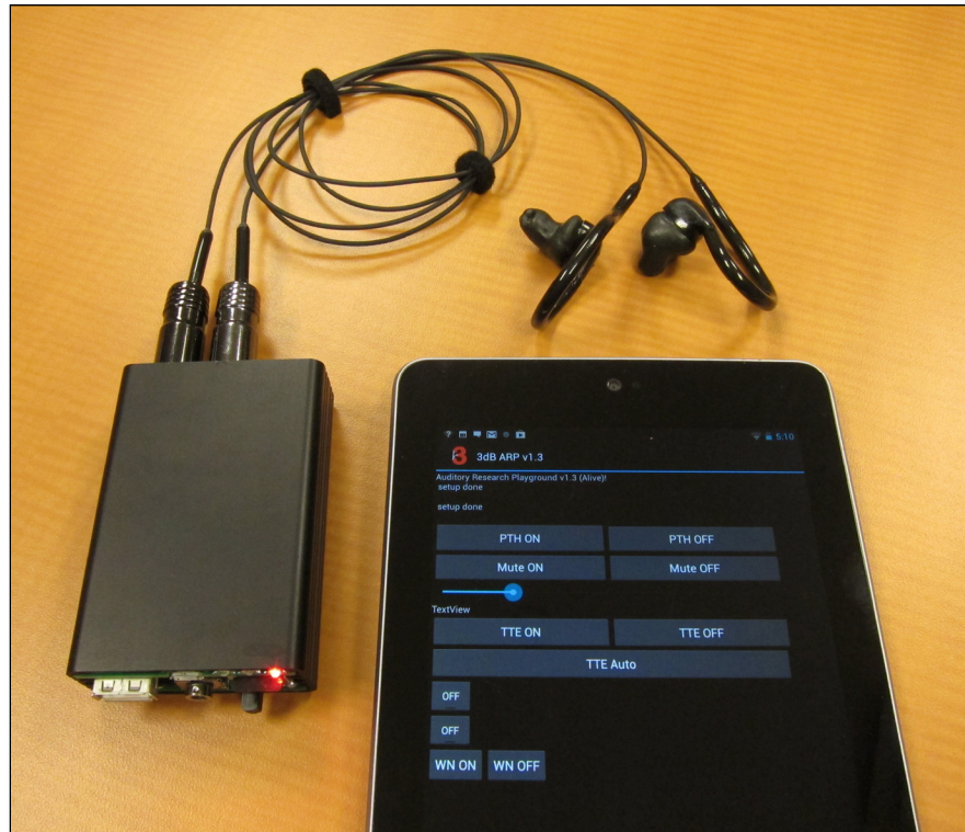
Figure 3.1 Photo of the completed ARP hardware interfaced to Android tablet
