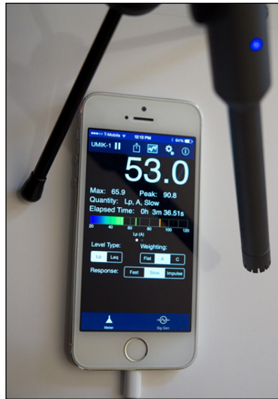
Figure 2.18 iPhone 5S running SoundMeter with the MiniDSP (Hong Kong) UMIK-1 connected via the 'Lighting to USB Camera Adapter'
