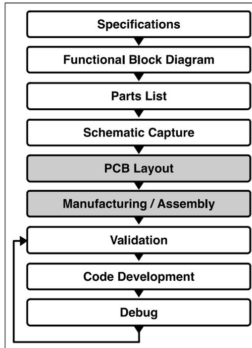
Figure 2.14 Overview of the flow of the ARP development and manufacturing process. The shaded steps (PCB layout and Manufacturing/Assembly) indicate steps outsourced to a local company
