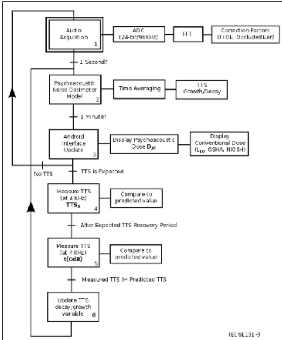
Figure 5.2 Sequential function chart of the proposed dose and recovery algorithms. Block 1 is the sampling of the noise signal using the earpiece microphones, Block 2 is the “Psychoacoustic Noise Dosimeter Model” (Kostek et al., 2012), Block 3 is the Android software interface, Block 4 and 5 represent the in-situ TTS measurement using the ARP hardware and Android interface to update the variables in the dosimeter model (2) on an individual basis
