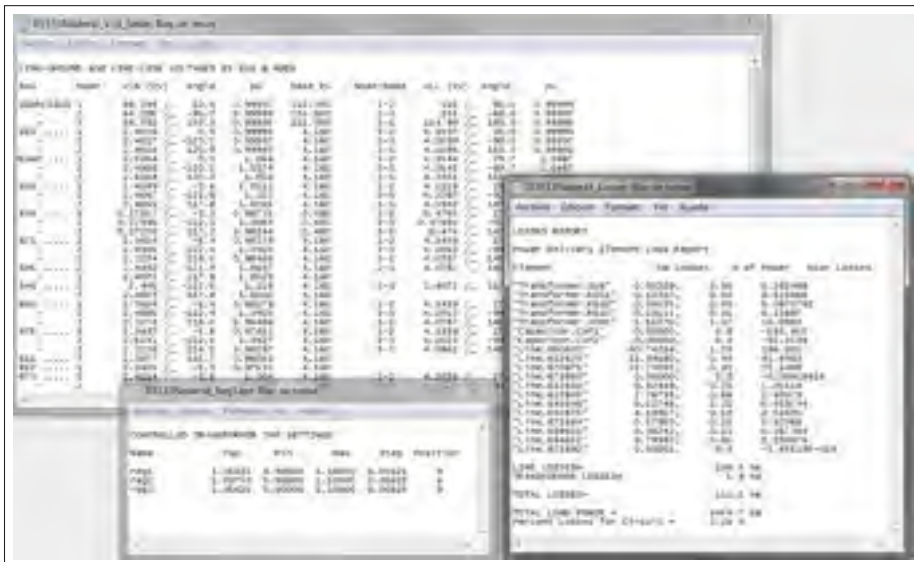
Figure 2.2 Node voltage, circuit losses and taps movements presented in text interface
