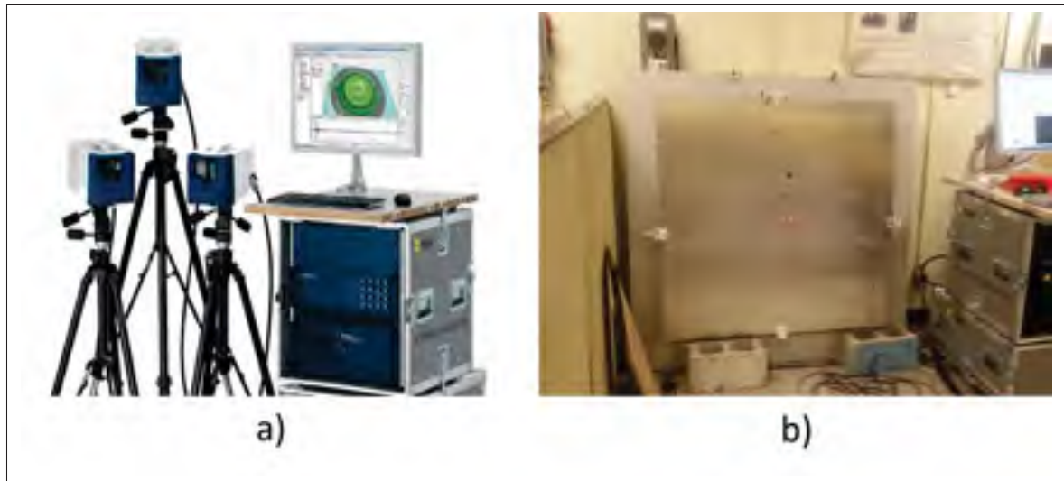
Figure-A I-5 a) Polytec PSV-500-3D, b) Experimental validation setup
