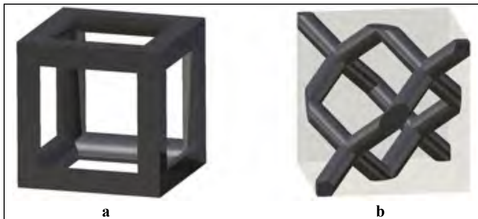
Figure 1.11 (a) Simple cubic and (b) diamond unit cells
