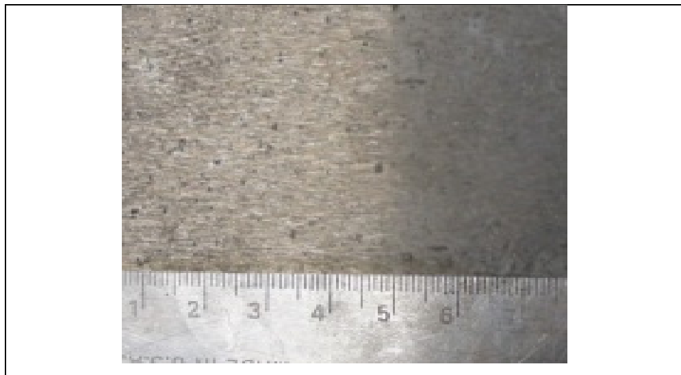
Figure 46 : Internal voids ( \sim 1\text{mm} ) observed from ingot cross-section.
