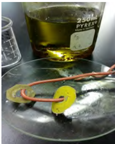
Fig. 5. The separated layers by the electrochemical process.
