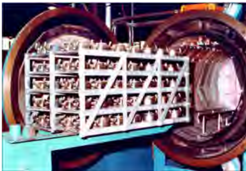
Figure 1-2 Fournaise de brasage (Brazing et Soldering, 2007a).
