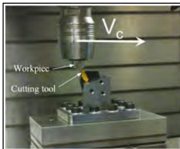
Figure 0-3 Orthogonal cutting configuration (Ducobu et al. , 2015)
