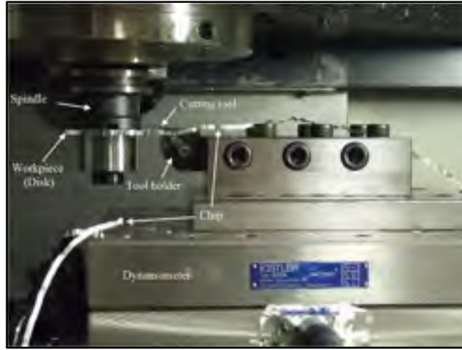
Figure 5-3 Experimental setup utilized during the orthogonal cutting tests
