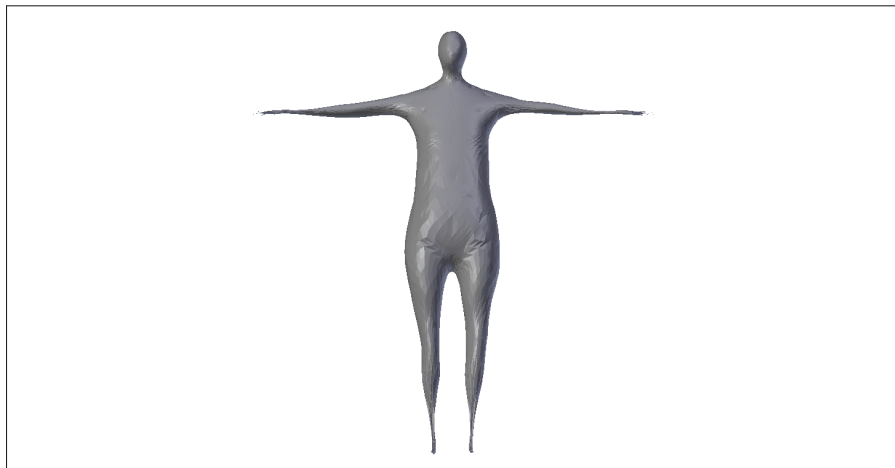
Figure 2.3 The source mesh after applying non-rigid registration. It deforms to match the faired target.
