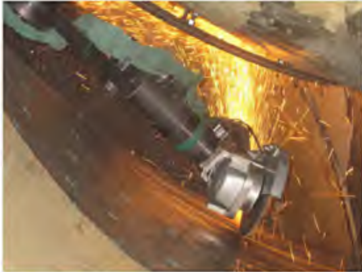
Fig. 8. SCOMPI robot performing grinding
