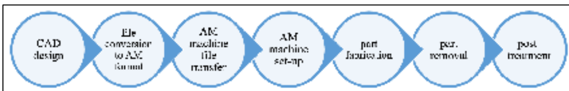
Figure 1.1 AM process flow (adapted from Gibson, Stucker and Rosen)
