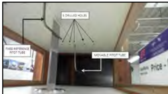
Figure 3.6 Test section calibration
