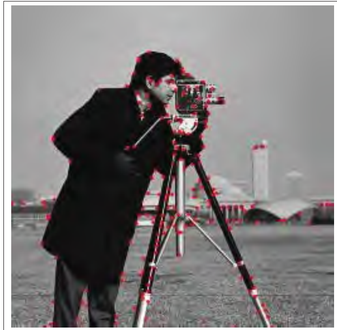
Figure-A II-1 Key points found using the Harris detector on the cameraman image.
