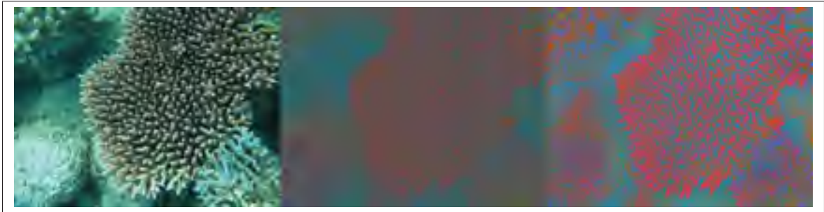
Figure 3.2 Comprehensive normalization preprocessing step example. From left to right: original image, comprehensive normalization output, additional adaptive histogram equalization for improved visualization.
