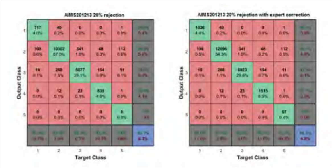
Figure 4.6 Confusion matrices obtained after rejecting the lowest 20% prediction scores (left) and after expert correction of the rejected samples (right) for AIMS2012-2013.
