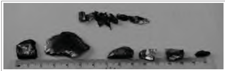
Figure 4.7 Chunks of metal found inside the main bearing of WT B.
