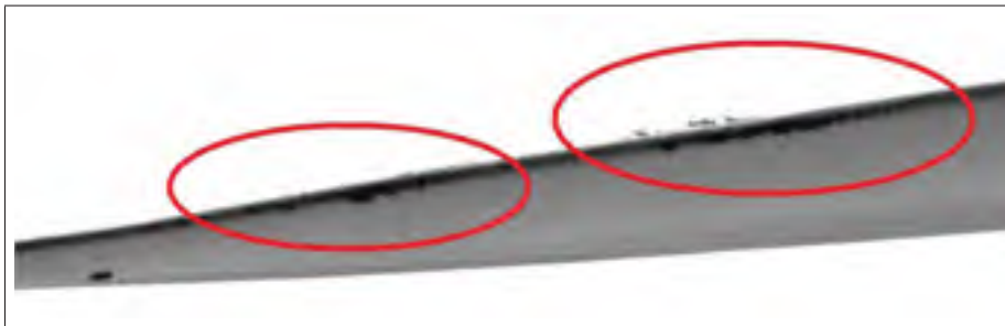
Figure 3.12 Picture of blade erosion taken in June 2013.
