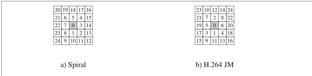
Figure 5.2 Subsets of the spiral search ordering (a) and the H.264 JM implementation of spiral search ordering (b). The gray square is the position of the MVP. Values in these grids show the evaluation order of candidate blocks (from 0 to 24).
