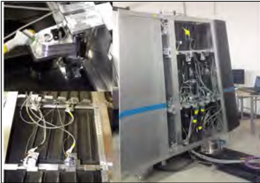
Figure 3.6 The wing-tip model with actuators and cabling system
