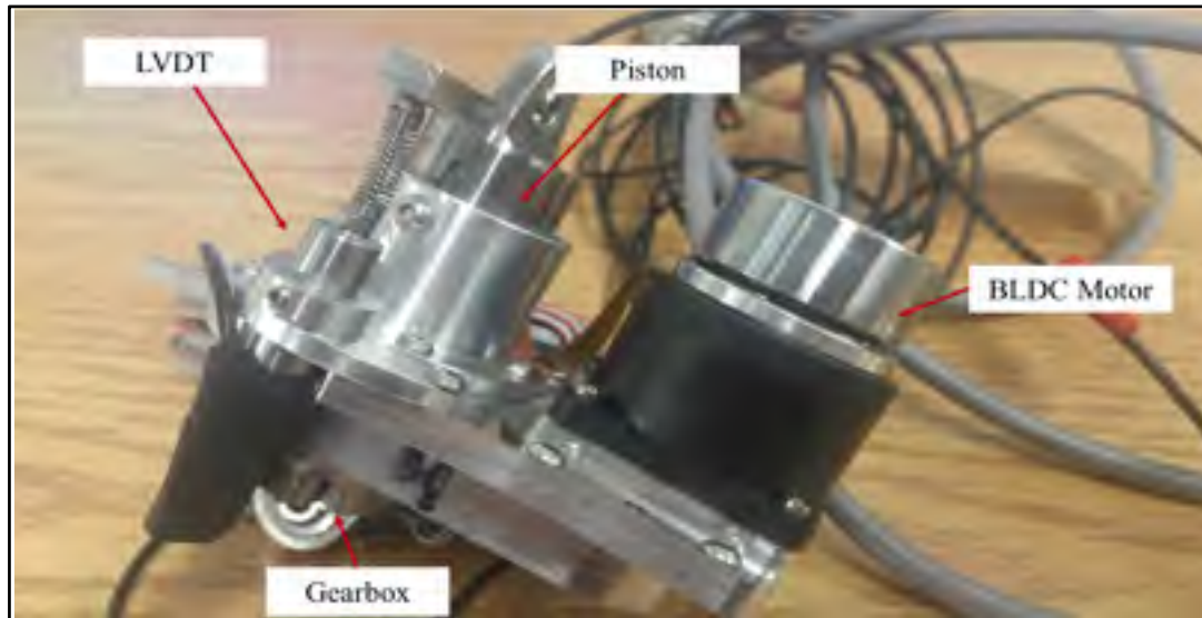
Figure 3.8 An actuator with LVDT sensors
