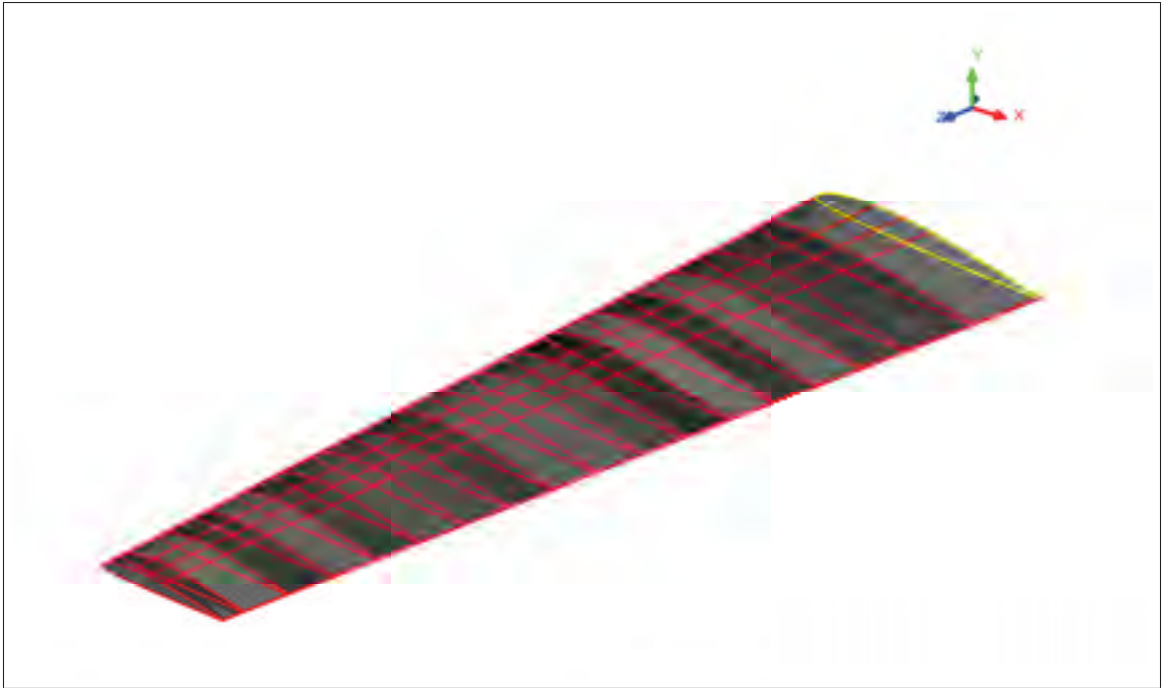
Figure 5.5 Quilted surface of a morphed wing
