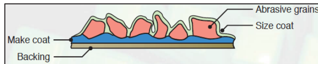
Figure 1.2 Grains sur un support (Kalpakjian, 2008)
