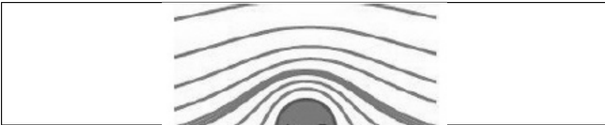
Figure 6.2 Schematic representation of velocity field as a result of traverse speed and rotational speed.
