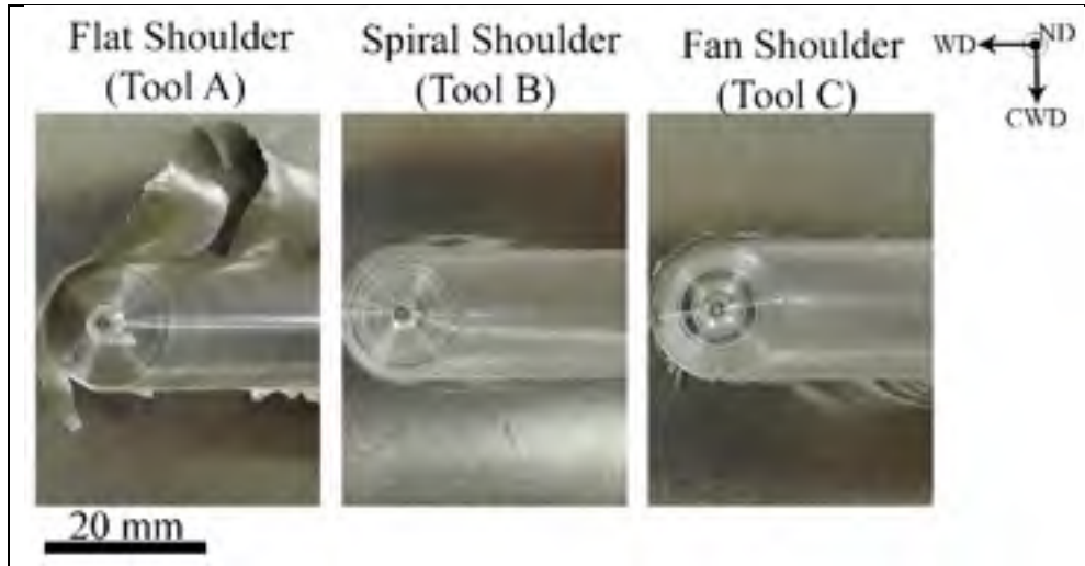
Figure 3.1 Surface morphology related to bead on plate of AA2024 material produced by tools A, B, and C. The spiral (tool B) and fan (tool C) shoulders prevent weld flashes.
