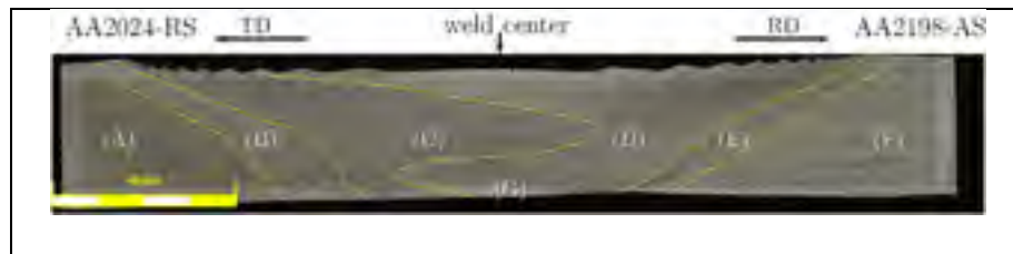
Figure 1.22 The macrograph of joint between AA2198 and AA2024 with higher magnification of different zones (Robe et al., 2015)
