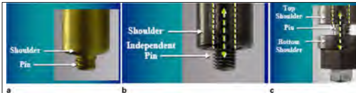
Figure 1.12 different types of FSW/P tools; a) fixed, b) adjustable and c) bobbin type tools (YN Zhang et al., 2012)
